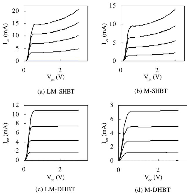
Figure 1. Common emitter characteristics of (a) LM-SHBT, (b) M-SHBT, (c) LM-DHBT and (d) M-DHBT ( $I_b=50\mu\text{A}/\text{step}$ )
