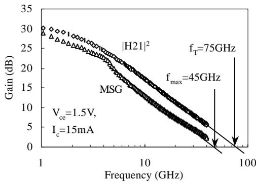
Figure 3. RF gains for a M-DHBT with  $5 \times 10 \mu\text{m}^2$  emitter
