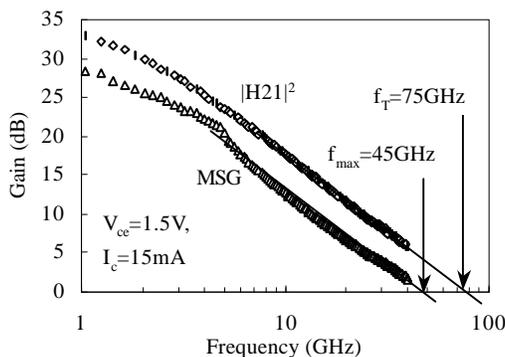
Figure 4. RF gains for a LM-DHBT with  $5 \times 10 \mu\text{m}^2$  emitter
