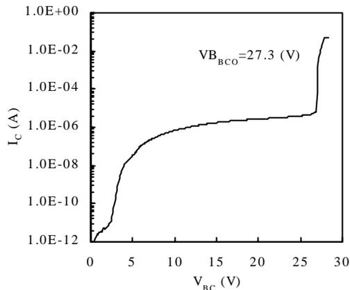
Fig. 6. Measured collector current as function of base/collector voltage for breakdown voltage testing of M-HBT (In<sub>0.15</sub>GaAs).
