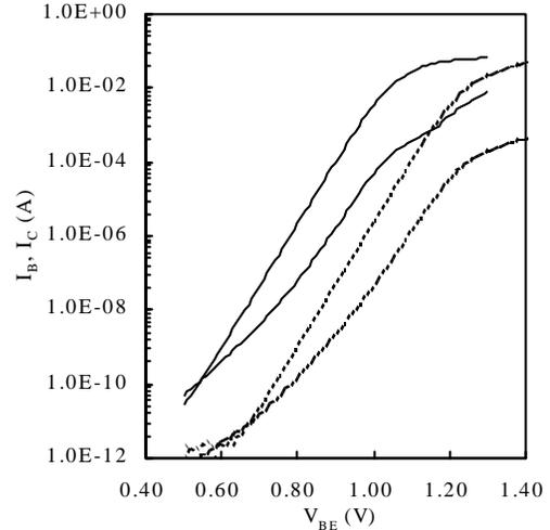
Fig. 3. Gummel plot for M-HBT with  $\text{In}_x\text{Ga}_{1-x}\text{As}$  base layer ( $x=0.15$ ) base layer and conventional InGaP-HBT with GaAs base layer. Large emitter area devices  $75 \times 75 \mu\text{m}$  were used for the D. C. testing.
