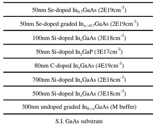
Fig. 1. Illustration of epi structure in HBTs. For conventional InGaP-HBT, x value in InGaAs layer is zero. For M-HBT, x values are 0.05, 0.10 and 0.15. Indium composition in InGaP emitter (y) is also raised so that it can lattice match to InGaAs base and collector.
