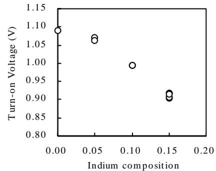
Fig. 4. Turn-on voltages in M-HBT as a function of indium composition ( $x$ ) in  $\text{In}_x\text{Ga}_{1-x}\text{As}$  base layer.  $V_{BE}$  at  $2\text{A}/\text{cm}^2$  collector current in  $75 \times 75 \mu\text{m}$  emitter area is defined as the turn-on voltage in this case.
