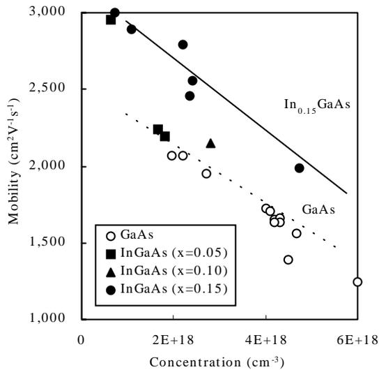
75×75μm emitter device, as a function of indium
