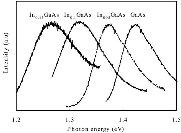
Fig. 2. Photo luminescence spectrum of GaAs and  $\text{In}_x\text{Ga}_{1-x}\text{As}$  ( $x=0.05, 0.1, 0.15$ ) subcollector layer.
