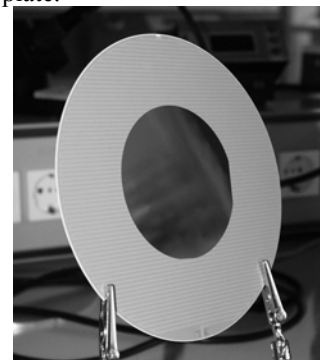
Figure 6: First demonstrator of an electrostatic support substrate: “Smart Carrier”, holding a 3” GaAs wafer.
