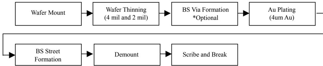
Figure 1 Standard 4-mil/2-mil 6-inch backside process
