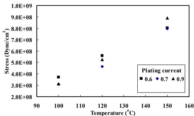
Figure 4 Plated Au film stress after thermal treatments
