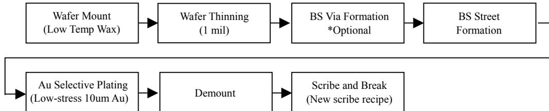
Figure 2 New 1-mil 6-inch backside process
