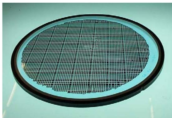
Figure 6 A completed 1-mil thick 6-inch wafer on UV-tape
