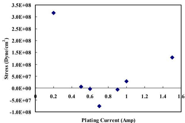
Figure 3 The effects of the plating current on the film stress
