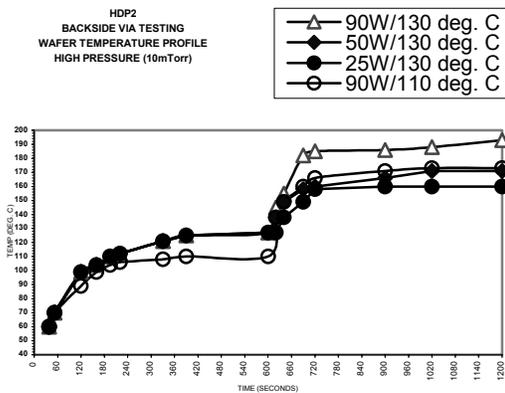
Figure 6. HBr-only chemistry with ICP power fixed at 900 Watts and chamber pressure at 10 mTorr.
