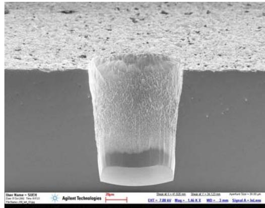
Figure 3. This is an example of a backside via in InP (etched in HBr-only). The photoresist mask has been removed. The sidewalls are fairly smooth with a square bottom profile. In this case, via depth is  $\sim 110\mu\text{m}$  and width at the bottom is  $\sim 80\mu\text{m}$ .
