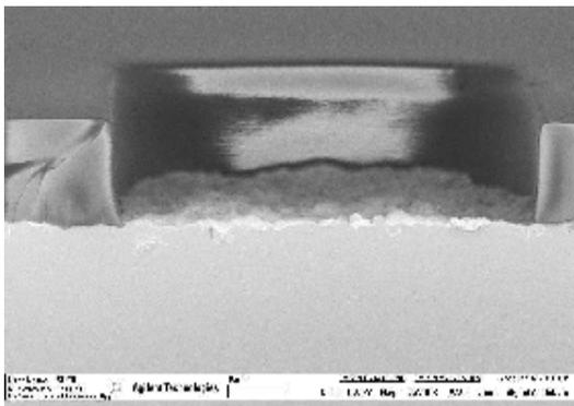
Figure 2. Micrograph of via feature (CD is  $70\mu\text{m}$ ) with the thick photoresist mask before the dry etch.
