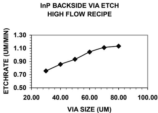
Figure 5. ARDE effects on etch rate.
