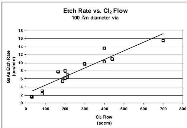
**Figure 4** Relationship between GaAs etch rate and Cl<sub>2</sub> flow over a range of pressures and RF powers.
