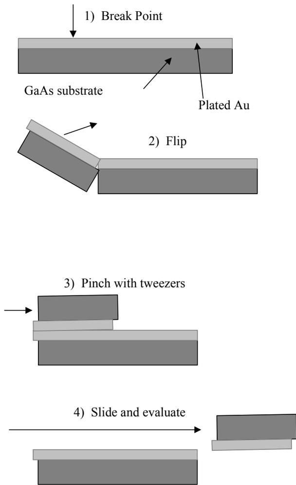
Figure 2: Break and slide method developed for adhesion evaluation.
