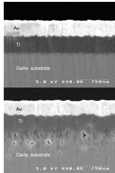
Figure 1: SEM cross-sections of 1:1 dilute (top) vs. concentrated chemistry (bottom). Note voiding at Ti-to-GaAs interface for the concentrated sample.
