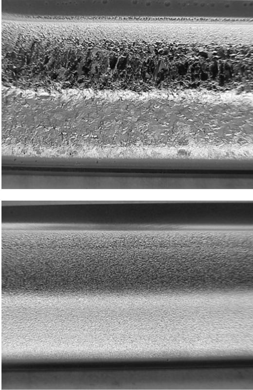
Figure 5: SEM images of large (top) and small (bottom) grain titanium targets.
