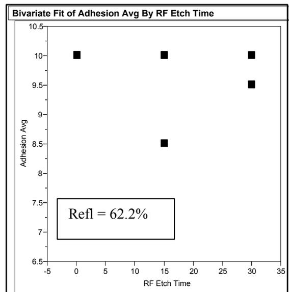
Figure 4: RF etch-GaAs surface reflectivity interaction. Note that for a sample with high reflectivity (top), correlation exists with RF etch time and for a surface with low reflectivity (bottom) no correlation exists.
