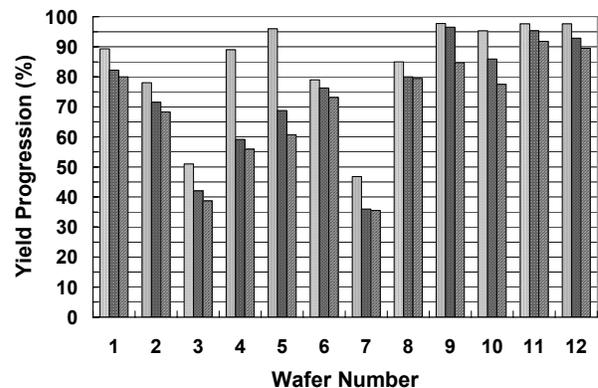
Figure 4. Illustrating parametric yield for individually grounded backside via holes, 1 mA/mm breakdown voltage (Vbdg1), and pinchoff voltage at 1 mA/mm drain current.
