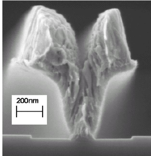
Figure 3. SEM cross-sectional view of a double-recessed self-aligned gate GaAs pHEMT device.
