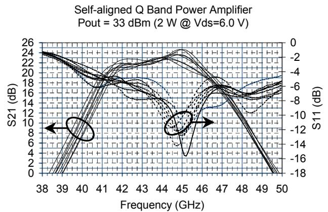
Figure 5. Illustrating the performance of a double-recessed, three-stage Q band power amplifier produced with the self-aligned process.
