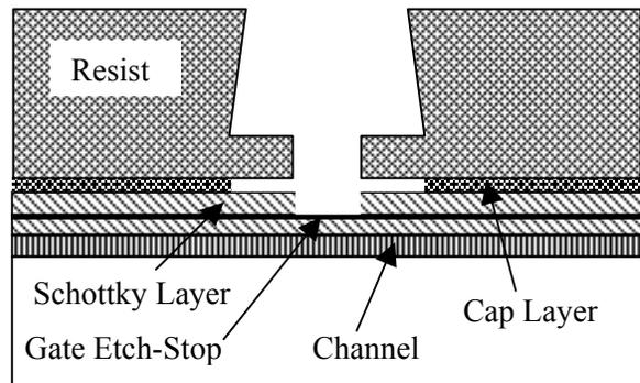
Figure 2. A generic cross-sectional schematic of a double-recessed and self-aligned pHEMT device.
