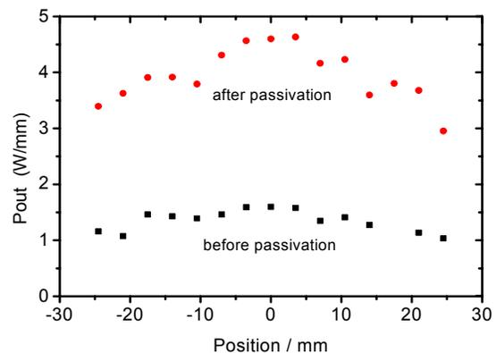
Fig. 2: Comparison of load pull power results before and after passivation for HEMTs at different radial position on the wafer. The gate width is  $100\ \mu\text{m}$ .
