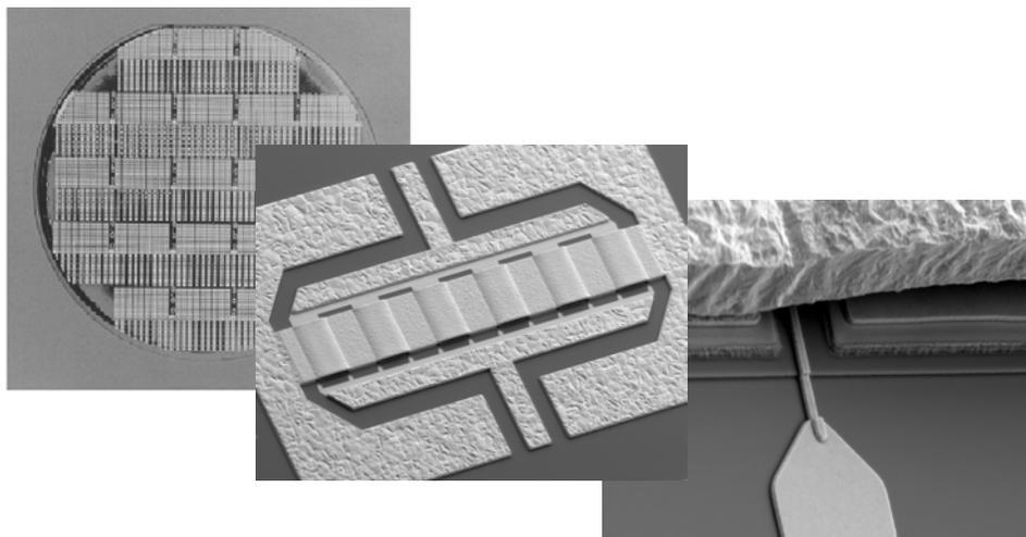
Fig. 1: AlGaN/GaN HEMTs on a 2'' wafer (left) comprising parallel transistor fingers (center) and detail of the gate feeding (right) also showing the transistor channel and arch of the air bridge structure.
