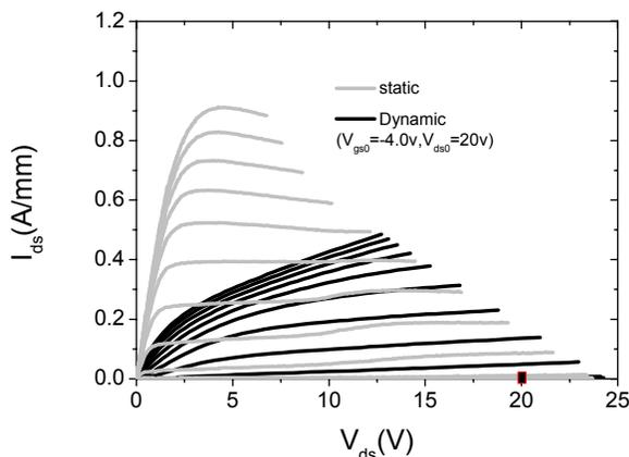
Fig. 3b: Comparison of static (—) and dynamic (—) output characteristics. Steady bias point for pulsed measurement:
