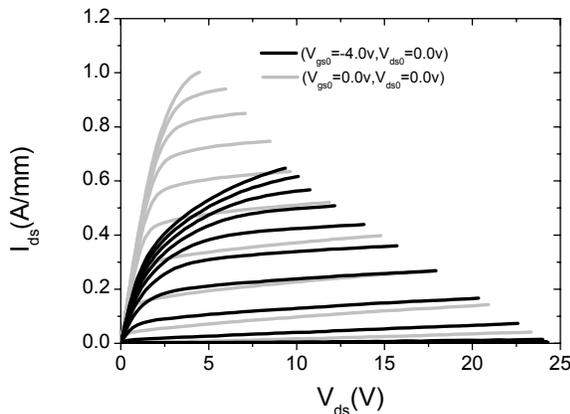
Fig. 3a: Pulsed measurement of I/V-characteristics:
