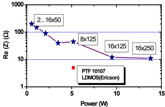
Fig. 4: Scaling of the output impedance with gate width at 2 GHz. The insets indicate the number of transistor fingers times finger width.
