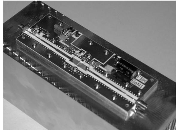
Fig. 5: Single stage amplifier with GaN-power HEMT output power in this configuration is 41,8 dBm (15,1 W) at 2 GHz.
