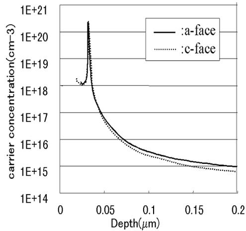
Fig.3 Comparison of C-V profile on a-face and c-face
