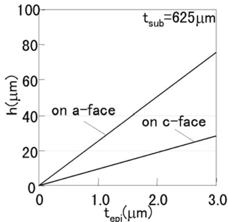
Fig.2 Calculated value of bowing
