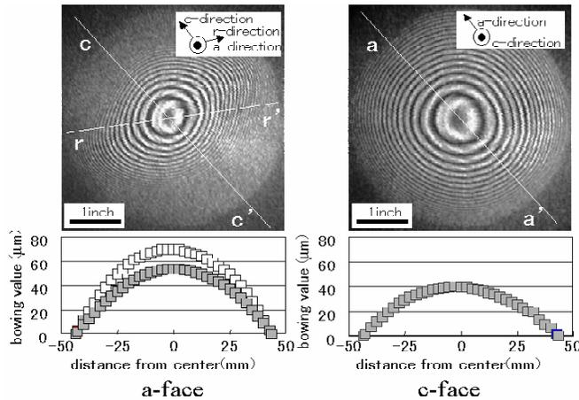
Fig.1 Bowing of 2μm GaN on 100mm diameter Sapphire
