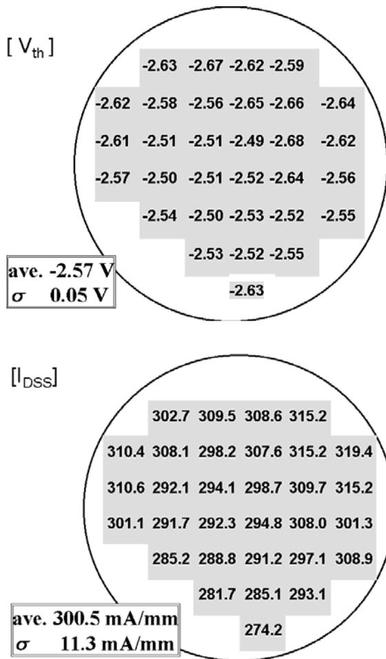
Fig.8 Uniformity of Ids at Vgs of 0V (Idss) and Vth across the wafer
