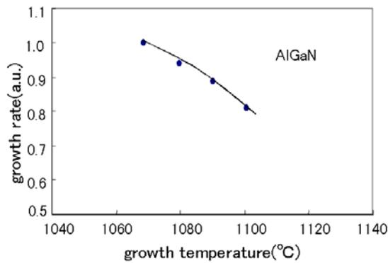
Fig.5 Dependence of growth ratio of AlGaAs and AlGaN on growth temperature
