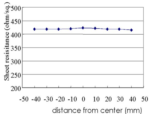
Fig.4 Uniformity of GaN-HEMT on 100mm substrate
