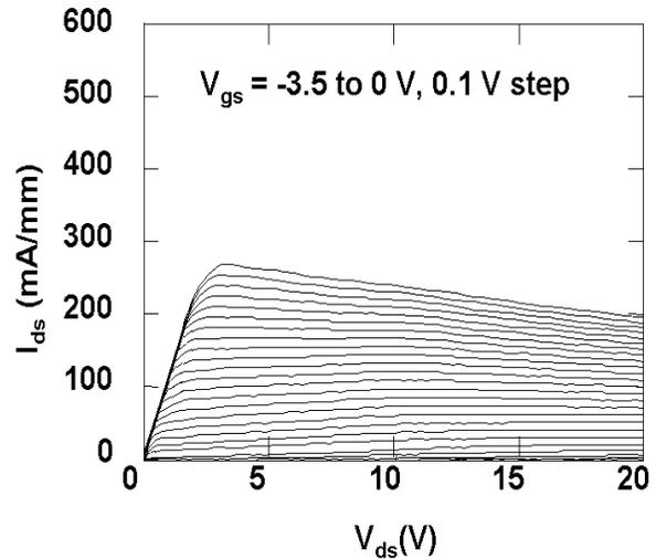
Fig.6 Ids-Vds Characteristics
