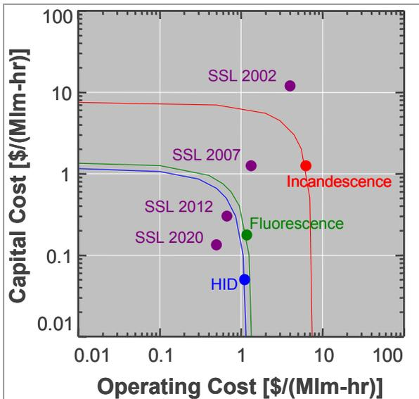
Figure 1: Graphical comparison of costs (ownership = capital + operating) associated with various white lighting technologies.
