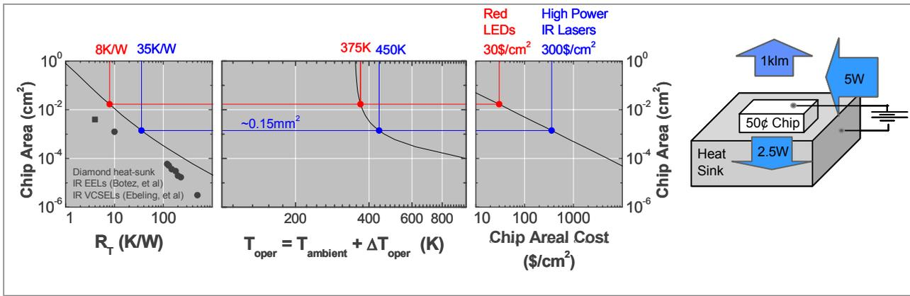
Figure 2: How chip areal cost and operating temperatures must scale with chip area in order to meet Roadmap targets.
