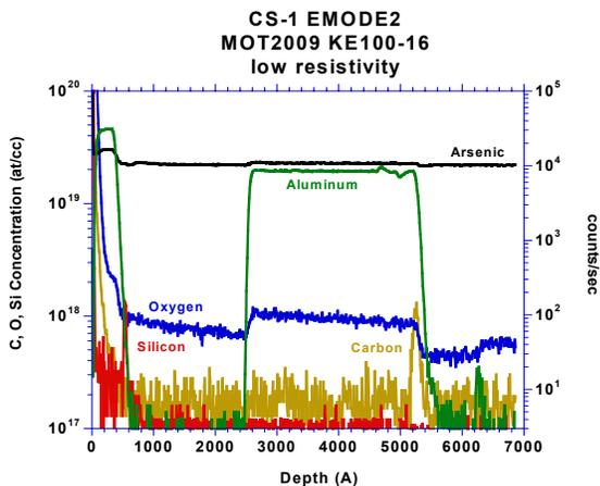
Figure 4 – SIMS data for a sample with a carbon pulse at the start of the buffer. Vt = 680 mV, FWHM = 30.8 sec<sup>-1</sup>. Sheet rho = 37,737 ohm/sq.
