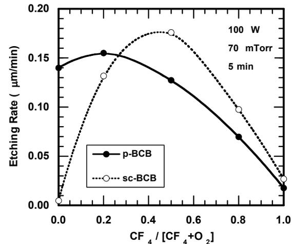
Fig. 3. Etching rate as a function of the CF<sub>4</sub>/O<sub>2</sub> gas ratio.
