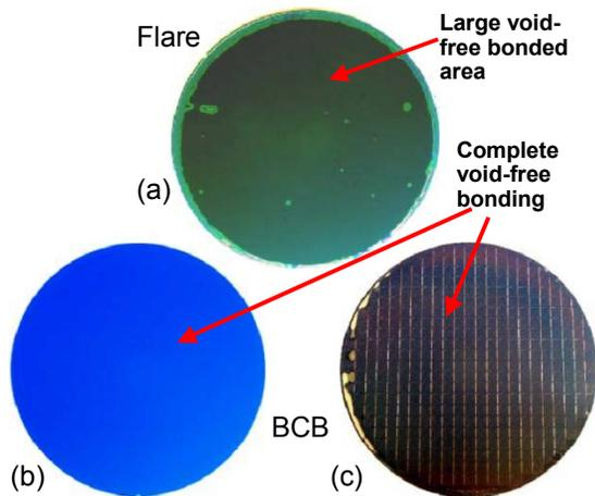
Fig. 3. Wafer bonding results [3]: (a) Corning glass 7740 bonded to Prime Si with Flare, (b) PG&O glass 1737 bonded to Prime Si with BCB, and (c) two via-chain patterned wafers bonded with BCB. No visible changes can be observed after Si wafers are thinned to  $\sim 30 \mu\text{m}$ .
