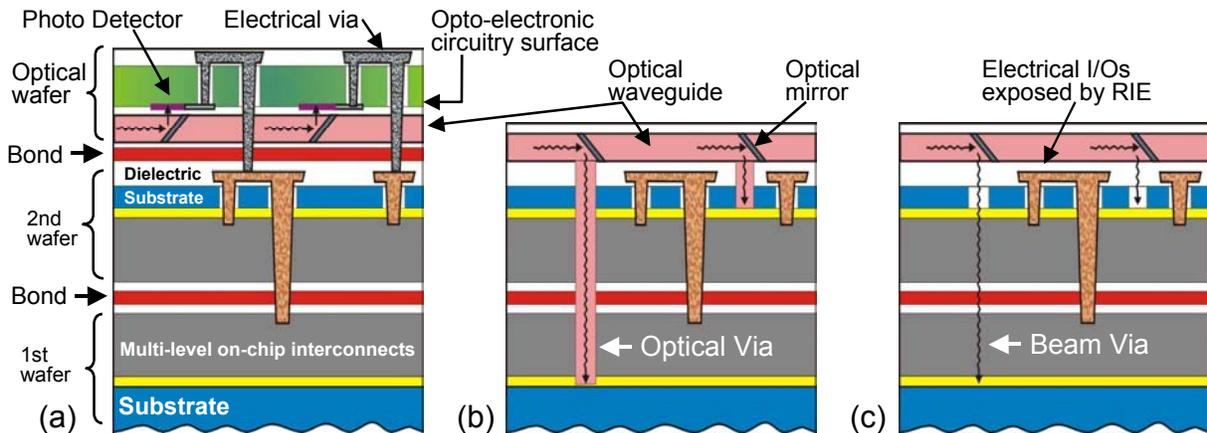
Fig. 7. Schematics of optical-electronic hyper-integration with (a) electrical vias, (b) optical waveguide vias and (c) optical beam vias.
