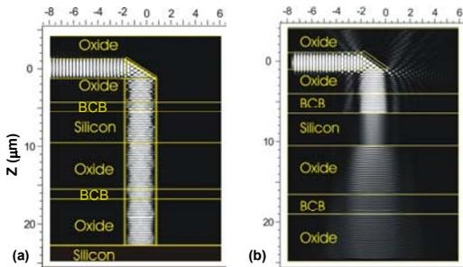
Fig. 8. Simulation result of the divergence of an optical beam through multilevel materials: (a) with an optical waveguide via filled by polymer with a refractive index of 1.51, and (b) without an optical via.
