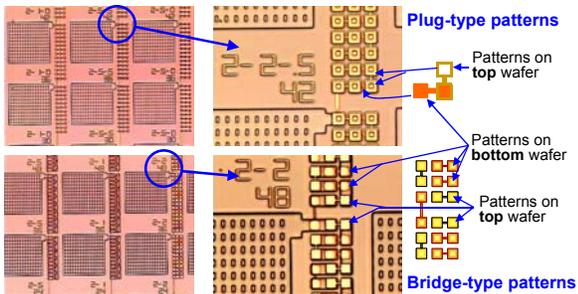
Fig. 6. 200 mm wafer-to-wafer alignment accuracy with via-chain test structures, indicating 1  $\mu\text{m}$  alignment can be achieved ( $<0.5 \mu\text{m}$  shown).
