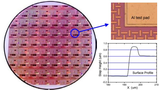
Fig. 4. Image of wafer with multi-level Cu-interconnects (provided by International SEMATECH) bonded on a glass wafer and backside thinned to  $35 \mu\text{m}$ . Right side: surface profile showing a step height of  $\sim 0.9 \mu\text{m}$  across the Al pads.
