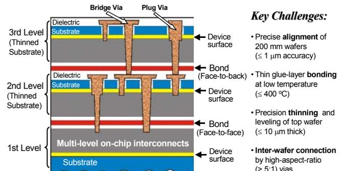
Fig. 2. Schematic of a hyper-integration 3D test vehicle using wafer bonding, showing bonding interface, vertical inter-wafer vias (plug- and bridge-type), and "face-to-face" and "face-to-back" bonding.
