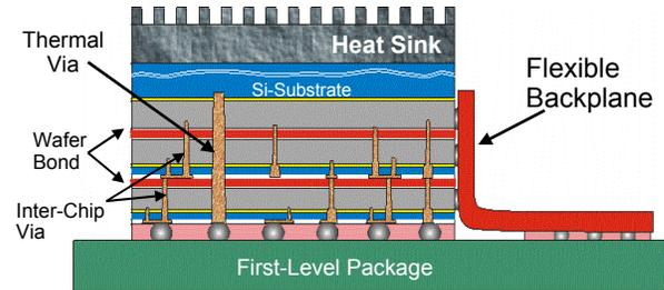
Fig. 9. Package assembly envisioned with hyper-integration technology. Thermal and ground vias enable cooling and electrical isolation; flexible backplane (edge contracts) offers additional I/O capability.
