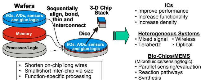
Fig. 1. Hyper-integration platform based on 3D vertical integration for future IC chips and heterogeneous systems, formed by monolithic wafer alignment, bonding, thinning and inter-wafer interconnection.
