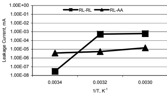
Figure 3 Temperature effect on TaN TFR leakage currents at 7 V.
