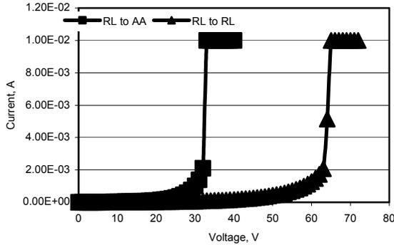
Figure 5 Breakdown voltage of both resistor to resistor and resistor to active area for TaN resistors, at 150 °C.
