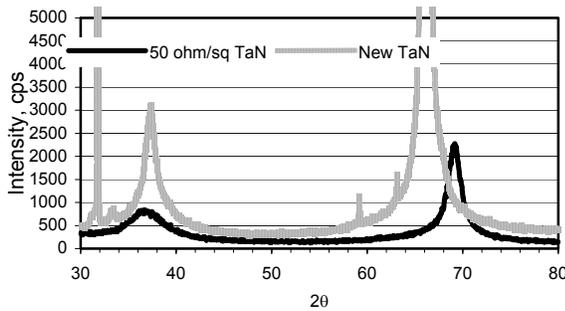
Figure 1 XRD comparison between the new TaN film and the 50 Ω/sq. TaN film, both on silicon substrates.
