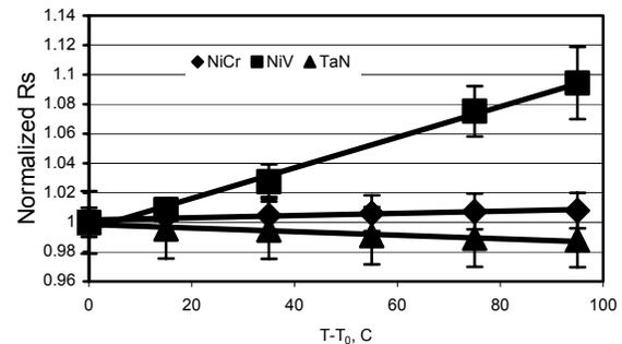
Figure 2 Temperature coefficient of resistance comparison for different TFR materials.
