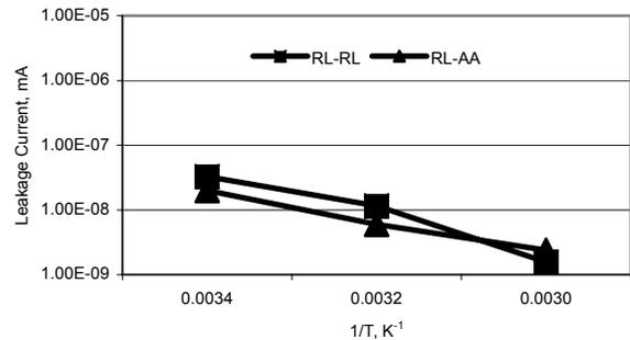
Figure 4 Temperature effect on NiCr TFR leakage currents at 7 V.
