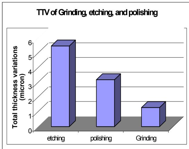
Fig. 1 shows the relationship between the total thickness variation (TTV) of the wafer finished with difference process. The polishing group has better flatness than the Wet etching. However, the grind-wafers have the best flatness in the wafer thinning operation, but its wafer strength is the lowest in the group as shown in Fig. 2.
