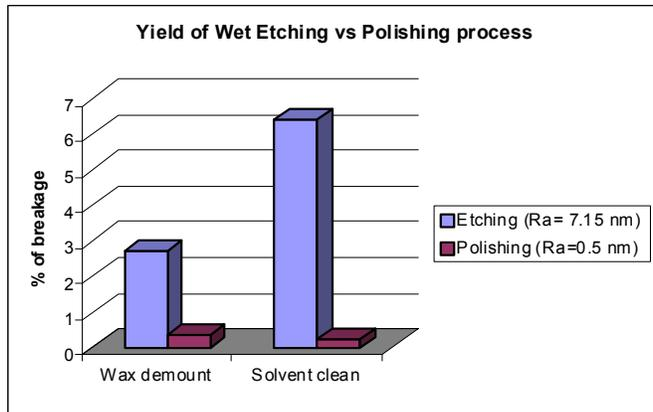
Fig. 4 shows the effect of the surface roughness and wafer yield. As the surface roughness value decreases from Ra=7.15 to Ra= 0.5 nm, the total wafer breakage rate decreased from 9.13% to 0.59%. Results from Fig.4 clearly confirm the importance of surface roughness in the yield. The polishing process can remove surface defects and reduce the surface roughness more effectively than the wet etching method.
