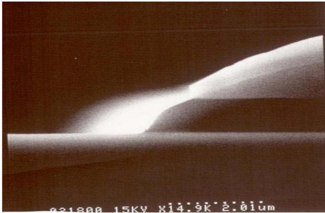
Figure 5. A SEM picture of BCB profile at low RIE power
