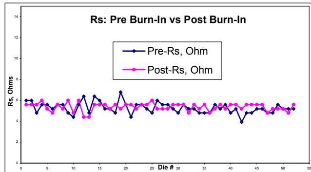
Figure 11. Rs before and after HTRB.
