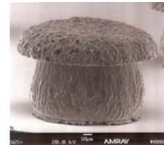
Figure 2. Before reflow. Figure 3. Pb-free before reflow.
