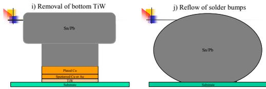
Figure 1. Schematic diagram of solder bump process.
