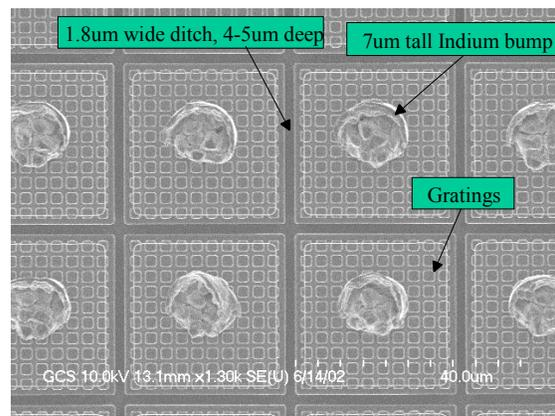
Figure 2(a). QWIP Top View SEM.
