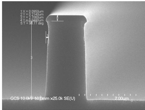
Figure 3(a) and (b). InP-based ridge waveguide device.
