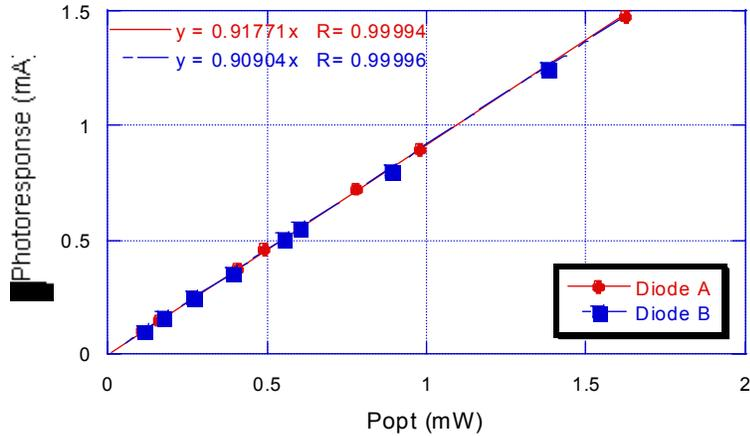
Figure 1(c). Responsivity: slope = 0.91 A/W at 1310nm.
