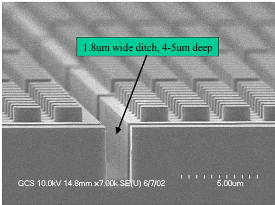
Figure 2(b). OWIP Cross Section.
