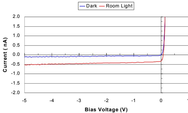
Figure 1(d). Dark current of InGaAs PIN PD.
