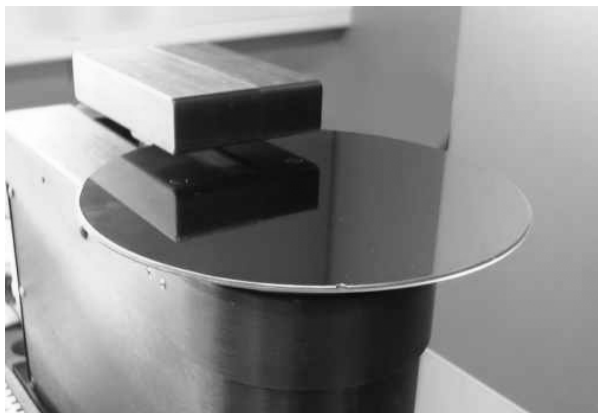
Fig. 5: Pre-alignment of III-V wafer and sapphire carrier.
