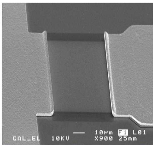
Figure 3-TaN resistor, SEM inspection
