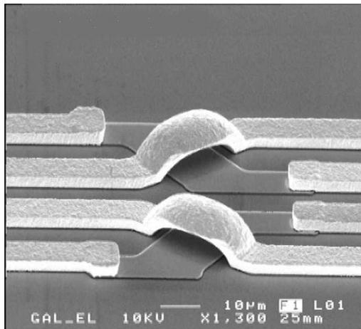
Figure 2-couplers, SEM inspection.
