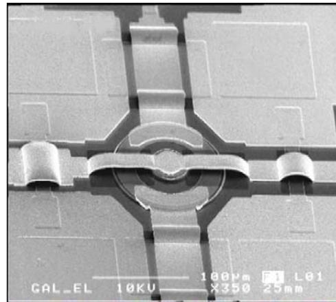
Figure 1–CPW diode, SEM inspection.
