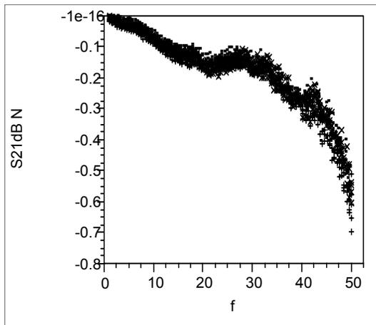
Figure 4 – 50 μm diode – Insertion Loss at -5 volts Reverse bias
