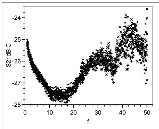
Figure 5 - 50 μm diode – Isolation at 20mA forward bias.
