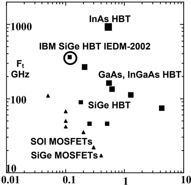
Fig. 1. Cut-off frequency of various transistors v. emitter/gate widths in  $\mu\text{m}$ .
