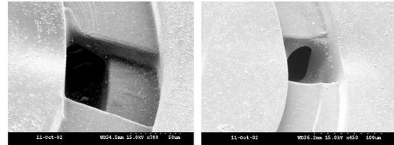
Fig. 3 Vertical vias detailed views. (80  $\mu\text{m}^2$ ).
