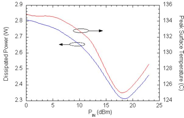
Fig. 2 Evolution of the peak surface temperature with the RF input power level.
