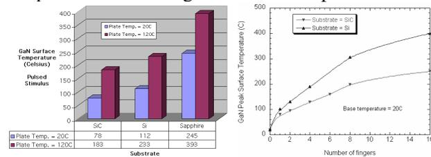
Fig. 2 Thermal simulation results.
