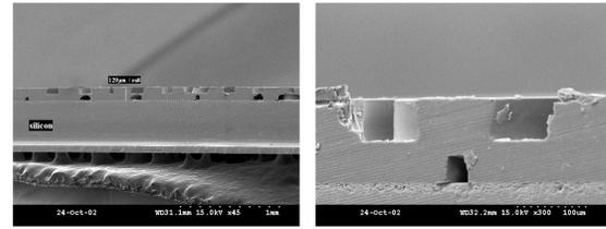
Fig. 3 Tri-dimensional micro-channel network cross-section view, and Stacked micro-channel detailed view.
