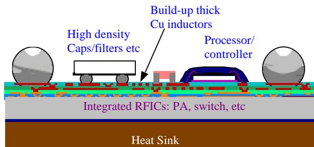
Fig. 4 Novel SiP scenario with overall integration
