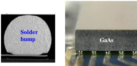
Fig. 2 GaAs wafer bumping and GaAs module assembly was implemented in ANADIGICS
