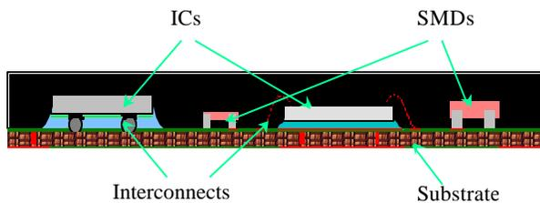
Fig. 1 Typical RF SiP platform
