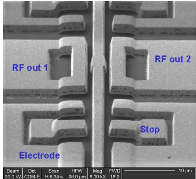
**Figure 2:** A scanning electron micrograph showing the center region of the LD switch.
