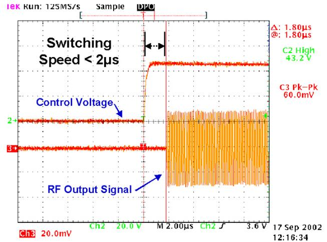
**Figure 5:** Switching speed of NGST's LD MEMS switch is less than  $2\mu\text{s}$  seconds under normal operation.
