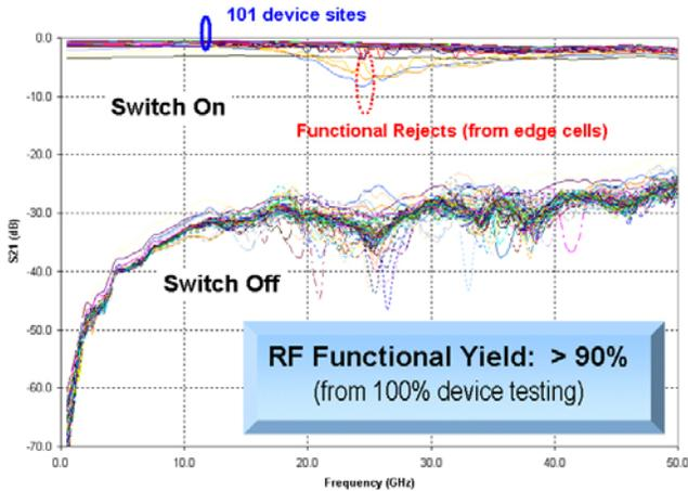
**Figure 7:** Representative RF data set from switches fabricated on a 100mm GaAs substrate showing excellent RF functional yield of the LD switches.
