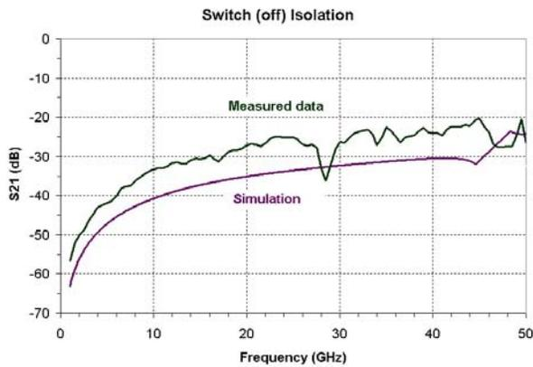
**Figure 4:** RF performance of the LD switch, Isolation of greater than 33dB at 10GHz, and 25dB at 50GHz.
