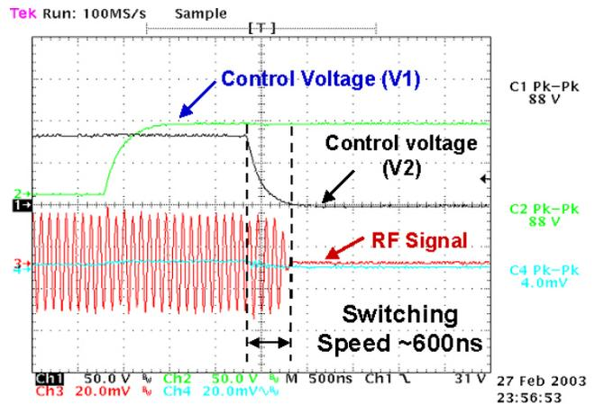
**Figure 6:** Sub-microsecond switching speed of the LD switch was demonstrated with “push-pull” operation.
