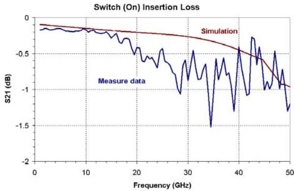
**Figure 3:** RF performance of the LD switch: IL of 0.2dB at 10GHz, and 1dB at 50GHz.
