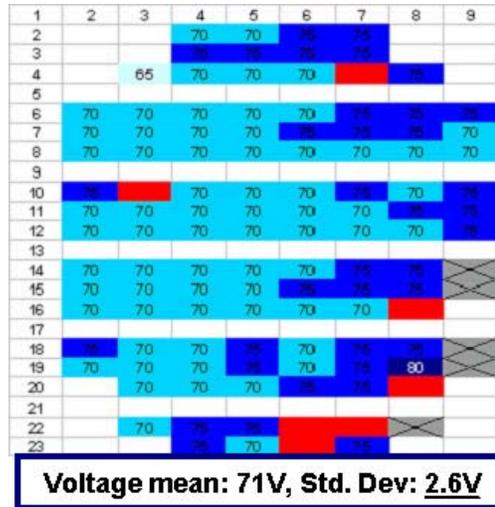
**Figure 8:** Actuation voltage map obtained from 100% testing of a 100mm GaAs wafer. The empty rows, (row 5, 9, etc) contain no switch devices, they are test cells with process monitoring structures. The cells with a cross denote incomplete cells in which the particular switch design under test is off the wafer edge.
