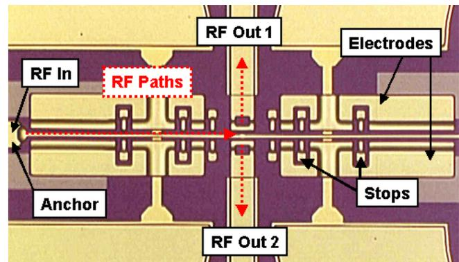
*Figure 1: Optical photograph of a lateral deflection RF MEMS switch showing its key features.*
