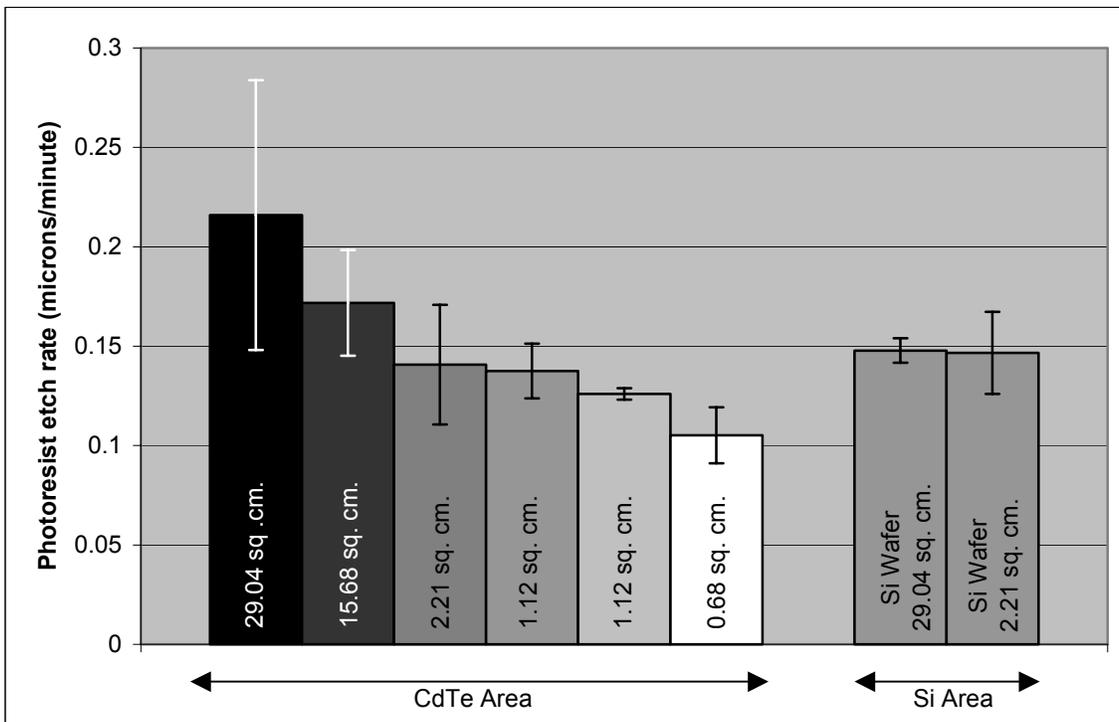
Figure 2. Photoresist etch rate as a function of semiconductor area. The photoresist etch rate increases with exposed CdTe area.
