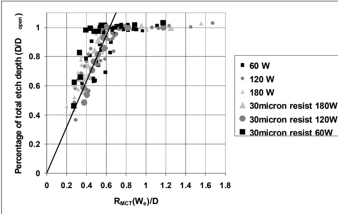
Figure 1. Trendline detailing the conditions necessary for the onset of etch lag for a variety of etching conditions.  $D/D_{open}$  is the ratio of the open area etch depth to the trench etch depth.  $R_{MCT}(W_e)/D$  is the ratio of the etch rate and trench width product to the open area etch depth.
