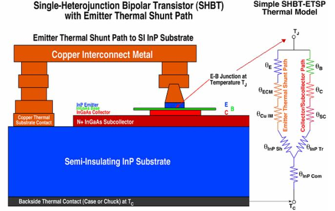
Fig. 4. Equivalent circuit and schematic cross section for emitter thermal shunt model.
