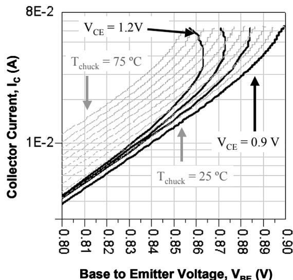
Fig. 1. Example thermal resistance measurement. Black lines represent room temperature measurements with  $V_{CE}$  fixed at values between 0.9 V and 1.2 V. The gray lines represent  $V_{CE} = 0.9 \text{ V}$  curves at chuck temperatures ranging from 25 to 75 °C.
