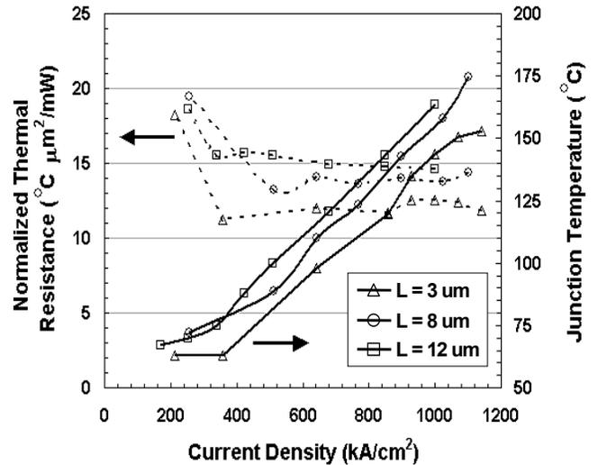
Fig. 3. Normalized RTH and  $T_j$  for UIUC75 SHBTs with lengths of 3  $\mu\text{m}$ , 8  $\mu\text{m}$ , and 12  $\mu\text{m}$ .  $W_E = 0.5 \mu\text{m}$  for all devices.
