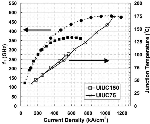
Fig. 2.  $f_T$  and  $T_j$  vs.  $J_C$  for collector thicknesses of 150 nm (squares) and 75 nm (circles) on  $0.5 \times 8 \mu\text{m}^2$  SHBTs.
