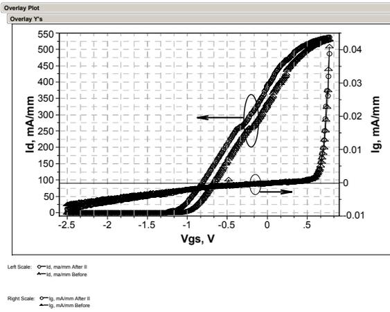
Figure 4.  $I_G$  and  $I_D$  as a function of  $V_{GS}$  before and after impact ionization stress. The triangles relate to the I-V characteristics before impact ionization
