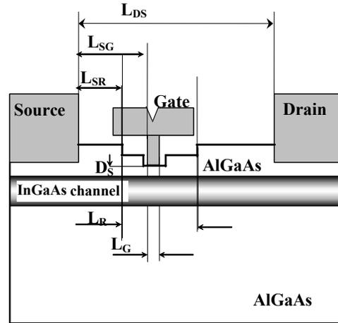
**Figure 1** Schematic diagram of the double-recessed PHEMT. The source-drain distance ( $L_{ds}$ ), source-gate distance ( $L_{sg}$ ), source-recess distance ( $L_{sr}$ ), recess width ( $W_r$ ), and gate length ( $L_g$ ) are layout parameters changed in the experiment are indicated. Their numerical values are given in Table I. Distance from the gate foot to the channel –  $D_s$  is the Schottky layer thickness.
