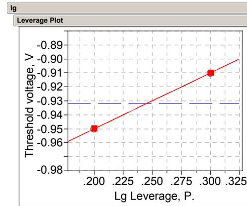
Figure 6a.  $V_T$  as a function of the gate length within the matrix before stress. The lines of 95% confidence coincide with the fitted line; dashed line presents the mean value.
