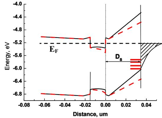
**Figure 3. Schematic view of the PHEMT energy bands dependence on distance from the gate. The dashed curve presents**
