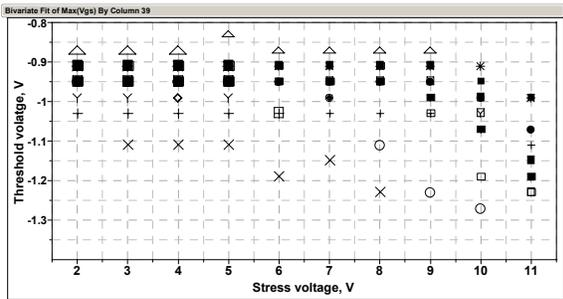
Figure 5. The threshold voltage for 16 devices of the Device Zoo as a function of the stress voltage applied at drain-source.
