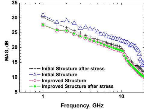
Figure 7 MAG as a function of frequency for two PHEMTs with identical layout and different vertical structure before and after stress.
