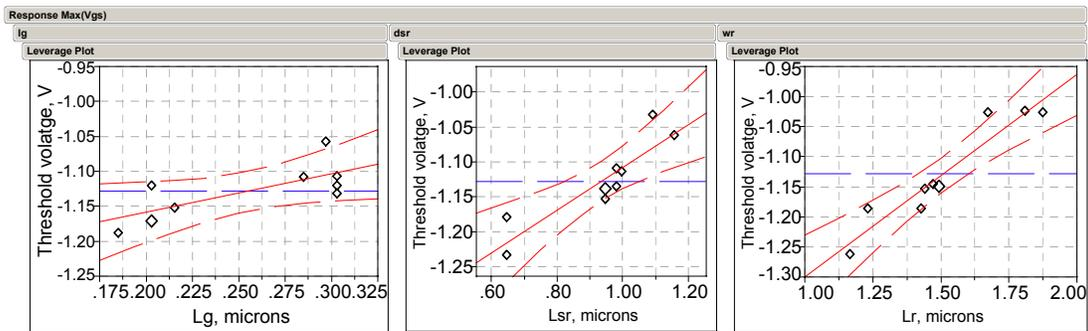
Figure 6b.  $V_T$  within the matrix after impact ionization stress at 10 V, as functions of  $L_G$ ,  $L_{SR}$ ,  $L_R$ . Red line is the function fitted to the experimental points. Dashed lines present the mean values. Long-dashed red lines are lines of 95% confidence in fitted line.
