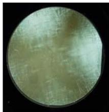
Fig. 1 Cross Polarized Image of 75mm Semi-Insulating SiC Substrate. Provided courtesy of II-VI Inc.
