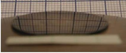
Fig. 2 25mm AlN Substrate. Provided courtesy of Crystal IS.
