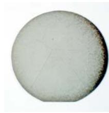
Fig. 2 50mm GaN Substrate. Provided courtesy of Kyma.
