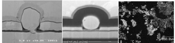
Figure 5 - Gold Defect Figure 6 – Gold Defect Figure 7 – Carbon Map
