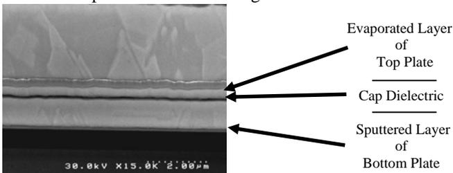
Figure 1 – Cross Section of HDMIM Capacitor
