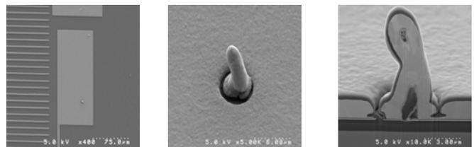
Figure 2 – Particle Resulting in Failing Capacitor
