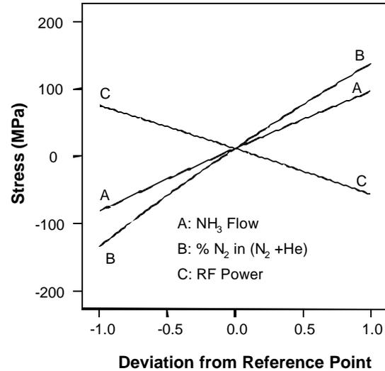
Figure 3. Perturbation effects on SiN<sub>x</sub> stress from factors, NH<sub>3</sub> flow, N<sub>2</sub>/He concentration, and rf power.
