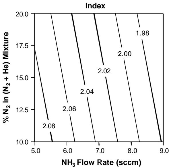
Figure 2. Refractive index as a function of NH<sub>3</sub> flow rate and N<sub>2</sub>/He concentration.
