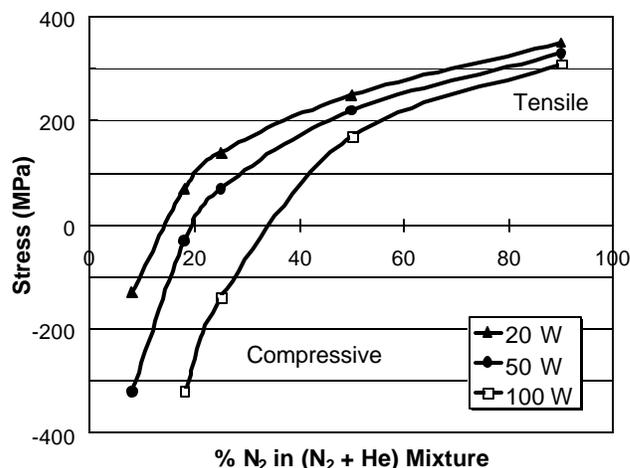
Figure 1. Stress control of PECVD SiN<sub>x</sub> by the He dilution method. The SiN<sub>x</sub> films were deposited at 250 °C at the different rf power levels indicated in the figure.
