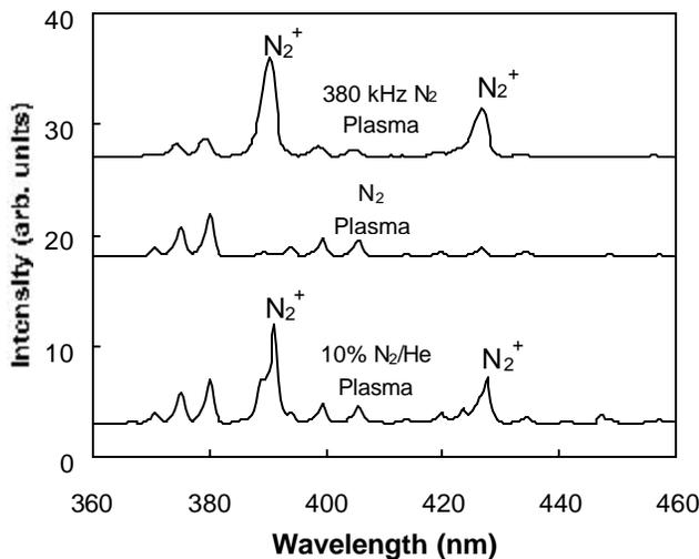
Figure 5. Optical Emission Spectra for 13.56 MHz plasmas of N<sub>2</sub> and 10 % N<sub>2</sub> in He. Also shown is a spectra of a low frequency, 380 kHz N<sub>2</sub> plasma. Spectra are displaced vertically for clarity.
