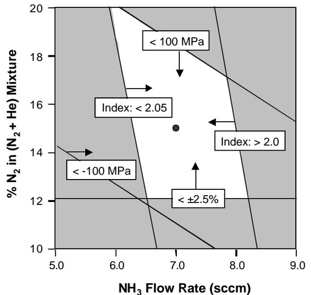
Figure 4. Overlay plot for an optimized low stress SiN<sub>x</sub> process. Non-shaded area shows the optimized process regime. Point in center denotes the center point of the design.
