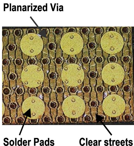
**Figure 4 – Backside solder bump technology made available by using epoxy planarized via technology**
