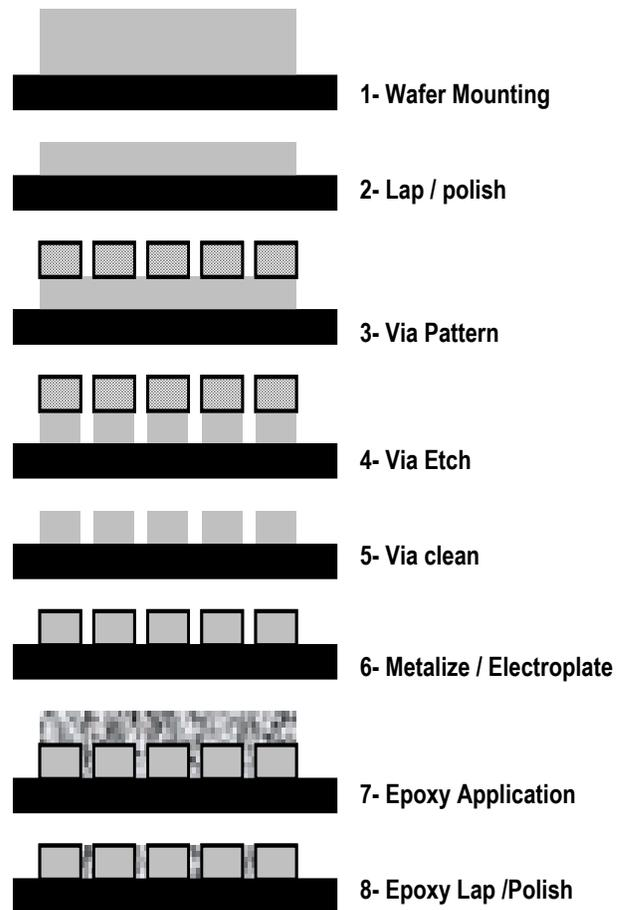
Figure 1- Schematic representation of the epoxy Planarization process
