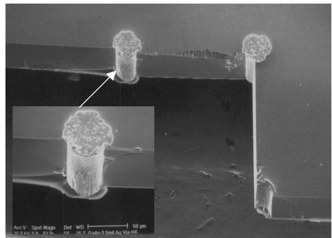
**Figure 3 – SEM photograph of solidly filled gold via structures in GaAs**
