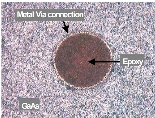
**Figure 2- Photograph of a 10 mils deep Epoxy planarized Via in GaAs**
