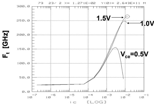
Figure 5.  $F_t$  versus  $I_c$  for an SHBT device similar to the DHBT in figure 5 above in terms of layout, size, epi layer and metal thicknesses.
