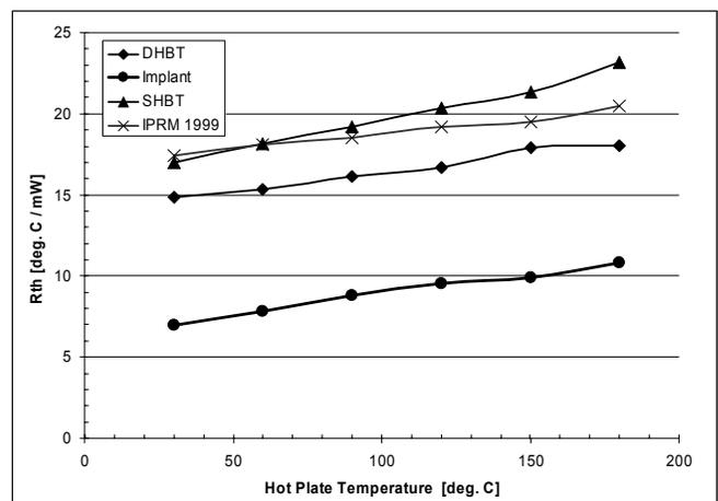
Figure 6. Thermal Resistance of InP HBTs from 30 to 180 °C measured at a constant emitter current density of  $250\mu A/\mu m^2$ .
