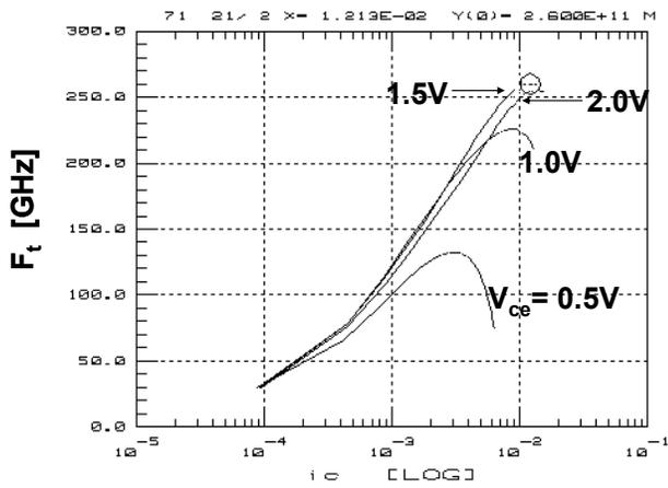
Figure 4. Unity current gain ( $F_t$ ) versus collector current for the DHBT device in figure 2 above.
