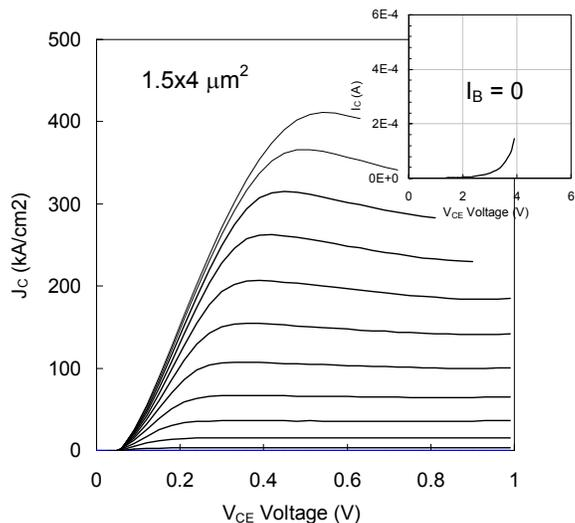
Fig. 5. Typical common-emitter IV characteristics of a  $1.5 \times 4 \mu\text{m}^2$  6.0 Å DHBT ( $I_{B\_STEP} = 50 \mu\text{A}$ )
