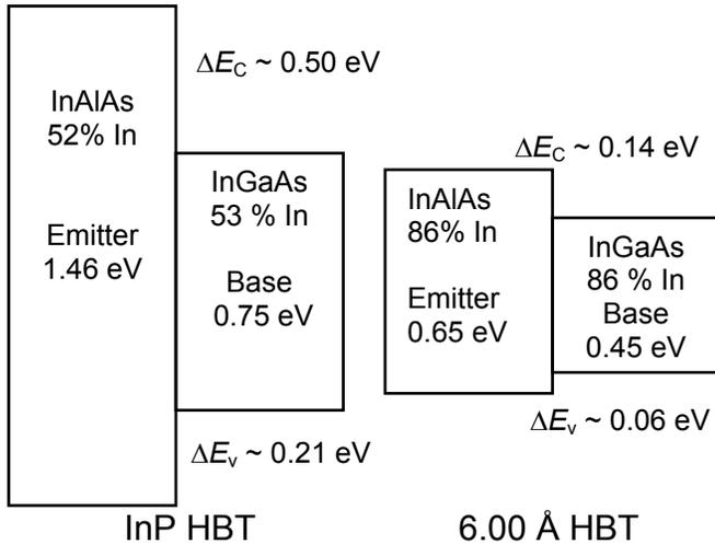
Fig. 2. Band line-up comparison between an InP-based HBT and this narrow-band-gap HBT material systems.
