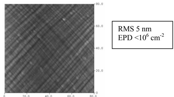
Fig. 1. AFM image from the surface of a In<sub>x</sub>Al<sub>1-x</sub>As metamorphic buffer graded in three steps (grown on InP substrate) terminating with 86 % Indium. The scan area is 80 μm x 80 μm
