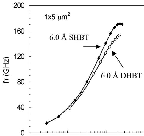
Fig.6. Cutoff frequency vs collector current density for a single (◆) and a double (◇) 6.0 Å HBT. The base-
