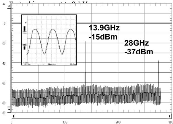
Fig. 7. Output spectrum of a divide-by-2 circuit operating at 28 GHz input frequency. The circuit uses 6.0 Å HBTs with emitter area of  $1.5 \times 4 \mu\text{m}^2$ .
