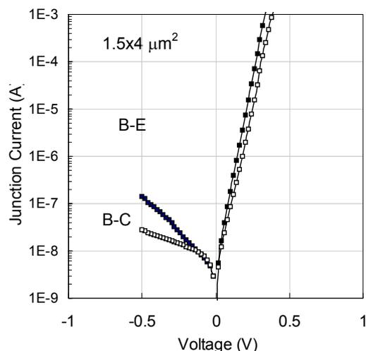
Fig. 4. Leakage current measured at collector-base and base-emitter junctions from a  $1.5 \times 4 \mu\text{m}^2$  narrow-band-gap HBT.
