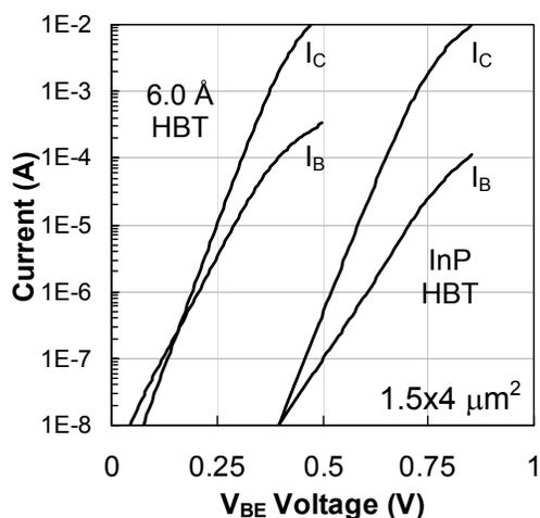
Fig. 3 Gummel-plot comparison between an InP-based HBT and an  $\text{In}_x\text{Al}_{1-x}\text{As}/\text{In}_x\text{Ga}_{1-x}\text{As}$  narrow band gap HBT using 86 % indium (6.0 Å)
