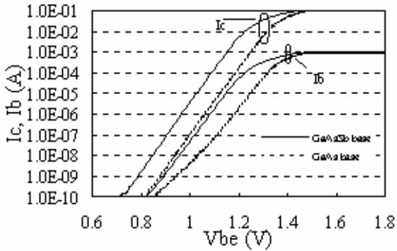
Figure 1. Small area device (15umx15um) Gummel plots of an InGaP/ GaAs<sub>0.93</sub>Sb<sub>0.07</sub> DHBT and an InGaP/GaAs HBT.
