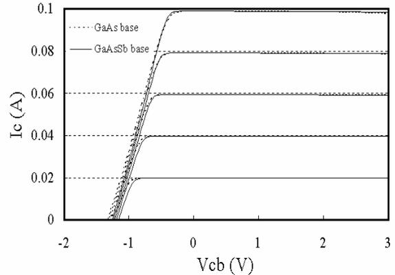
Figure 3. Common base I-V curves of a small area device (15umx15um) InGaP/GaAs<sub>0.93</sub>Sb<sub>0.07</sub> DHBT and an InGaP/GaAs HBT, the step of emitter current were 20mA.
