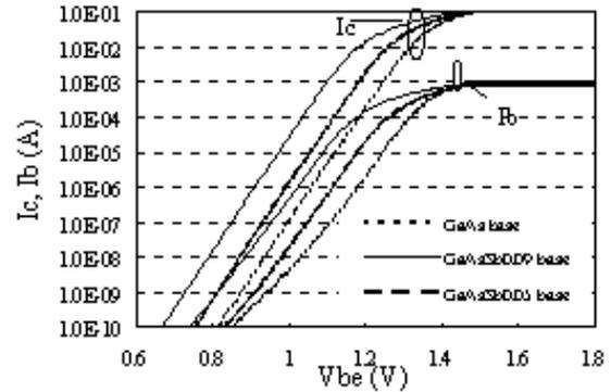
Figure 5. Small area device ( $15 \mu\text{m} \times 15 \mu\text{m}$ ) Gummel plots of an InGaP/ GaAs<sub>0.95</sub>Sb<sub>0.05</sub> DHBT, an InGaP/ GaAs<sub>0.91</sub>Sb<sub>0.09</sub> DHBT and an InGaP/GaAs HBT.
