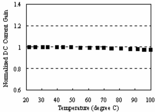
Figure 4. Normalized DC current gain versus temperature of an InGaP/ GaAs<sub>0.93</sub>Sb<sub>0.07</sub> DHBT.
