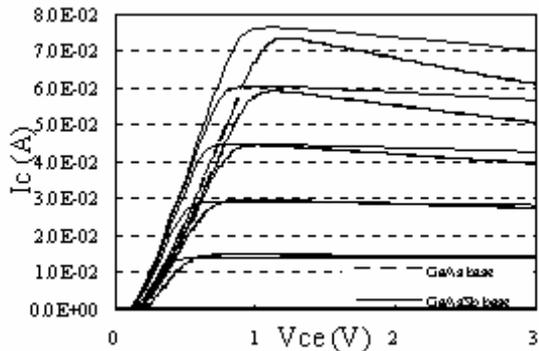
Figure 2. Common emitter I-V curves of a small area device (15umx15um) InGaP/ GaAs<sub>0.93</sub>Sb<sub>0.07</sub> DHBT and an InGaP/GaAs HBT.
