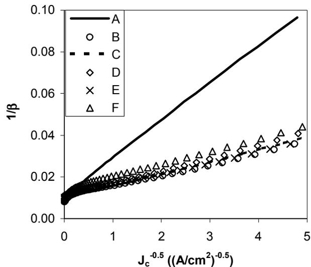
Figure 2. Base and EB junction components extracted from the stabilized Gummel traces of the six samples. The slopes are proportional to  $J_{scr}$  and  $J_{sr}$ . Intercept correlates to  $J_{abr}$ . ( $L=4 \times 20 \mu\text{m}^2$ )
