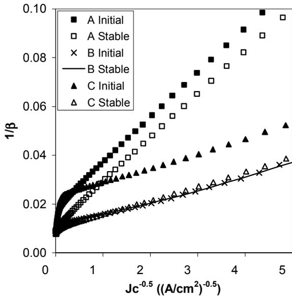
Figure 3. Base and EB junction components extracted from the initial and stabilized Gummel curves from devices A, B, and C. Slopes do not change during the burn-in stabilization. Linearly extrapolated Y-Intercepts from initial IV sweep of samples A (37% BI) and C (49% BI) are higher than Y-intercepts from stabilized devices. Sample B (3 % BI) shows very little shifts after the burn-in. ( $L=4 \times 20 \mu m^2$ )
