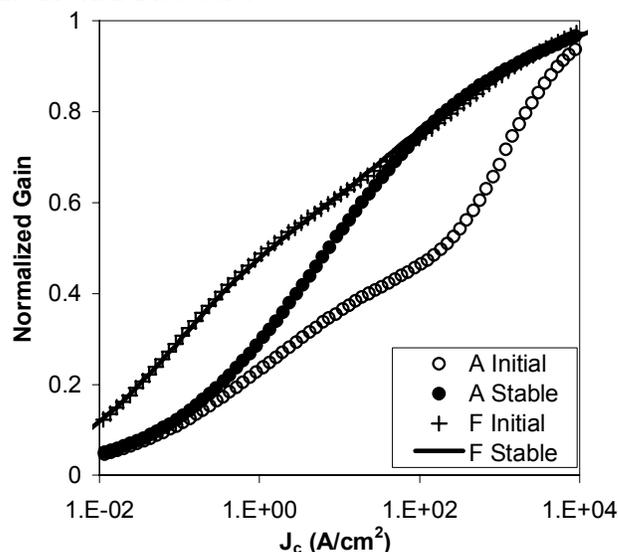
Figure 1. Normalized DC current gain transients of sample A and sample F. Samples A and F show 37% BI and 3% BI, respectively. ( $L=4 \times 20 \mu\text{m}^2$ )
