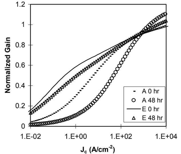
Figure 4. Normalized DC current gain of samples A and E after stressing at  $T_j = 210^\circ C$  and current density,  $12.5 \text{ kA/cm}^2$  for 48 hours. DC current gain shift at  $200 \text{ A/cm}^2$  for Samples A and E are  $-13\%$  and  $-1\%$ , respectively. DC current gain shift at  $12.5 \text{ kA/cm}^2$  for Samples A and E are  $12\%$  and  $6\%$ , respectively. ( $L = 4 \times 20 \mu m^2$ )
