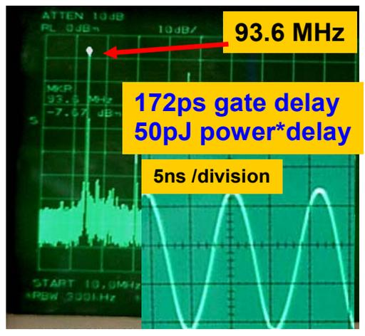
Figure 5 Frequency and time domain output of the 31-stage ring oscillator.
