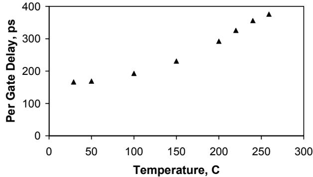
Figure 6 Plot of per-gate delay as a function of base plate temperature.
