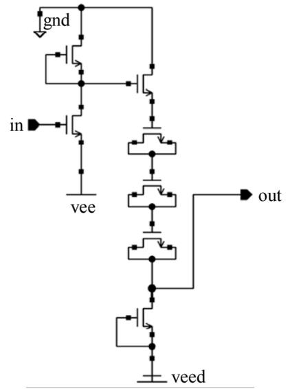
Figure 4 Schematic diagram of the inverter block used in the 31-stage ring oscillator.
