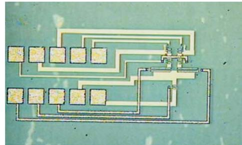
Figure 1 Micrograph of a GaN HFET comparator circuit.
