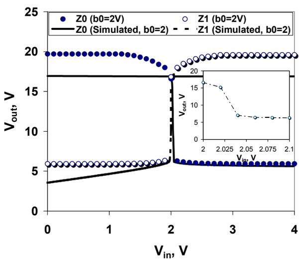
Figure 3 Measured and simulated transfer curves of the GaN comparator circuits.
