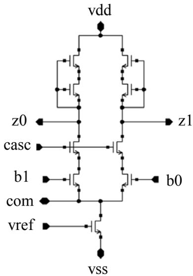
Figure 2 Schematic diagram of the comparator circuit.
