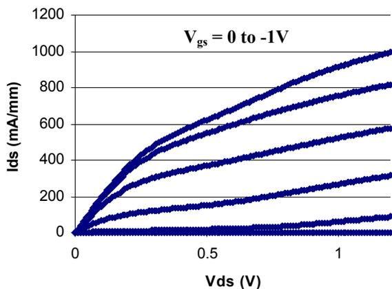
Fig 7. 70nm  $I_{\text{ds}} - V_{\text{ds}}$  device characteristics with threshold voltage  $\sim -0.85\text{V}$   $V_{\text{gs}}$
