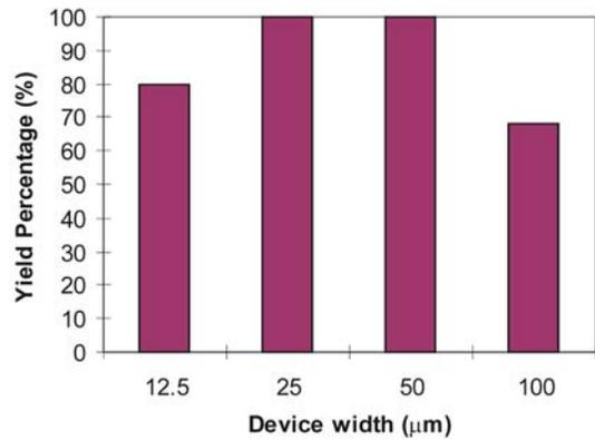
Fig 4. Measured device yield vs. device width
