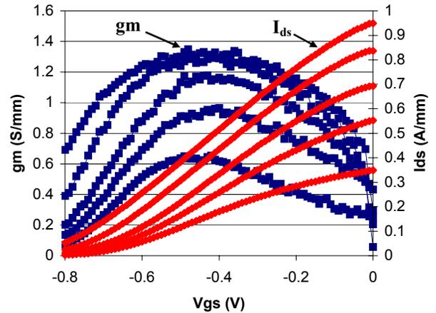
Fig 8. 70nm transfer ( $I_{\text{ds}}$ ) and transconductance ( $g_m$ ) characteristics for stepped source-drain bias  $0.2$  to  $1\text{V}$   $V_{\text{ds}}$ .
