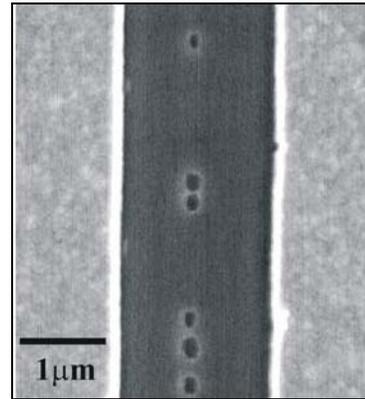
Fig 1. Patchy gate recess etch between source - drain metallisation
