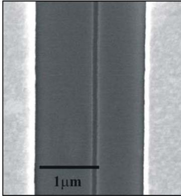
Fig 6. Clear gate recess etch between source - drain metallisation
