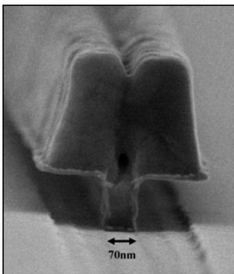
Fig 3. Metallised 70nm T-gate with double recess etch
