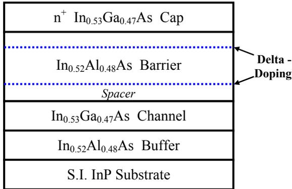
Fig 2. Double delta doped InP HEMT material structure
