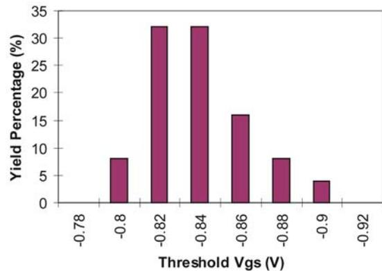
Fig 5. Threshold voltage distribution
