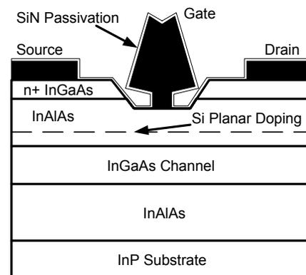
Figure 1. Cross-section diagram of an InGaAs/InAlAs/InP HEMT for low noise amplifier applications.
