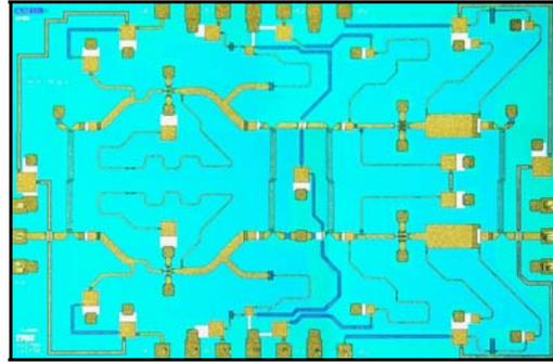
Figure 8. Micrograph of a Ka-band 2-staged balanced MMIC LNA operating over 27-39 GHz fabricated by 0.1  $\mu\text{m}$  InP HEMT technology on 100 mm InP substrate.
