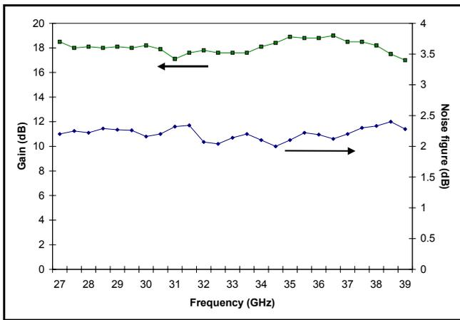
Figure 7. Noise figure and associated gain of a 0.1  $\mu\text{m}$  InP HEMT Ka-band 2-stage balanced LNA fabricated on 100 mm InP substrate.
