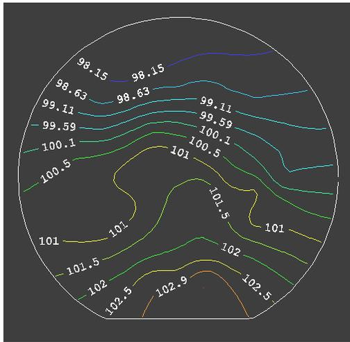
Figure 2. Resistivity plot for the 3 x 4-inch platform, showing excellent uniformity of 1%.
