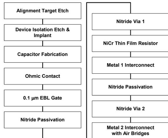
Figure 3. 100 mm 0.1μm InP HEMT Frontside fabrication process flow diagram.
