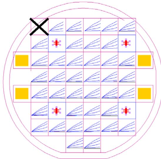
Fig. 6 Device yield of forty 4 x 75-μm devices across a 3" wafer depicted as location dependent DC-IV plots. Also drawn are four large-area hall bar, and four plating clip dropouts, and non-functional devices as "X".
