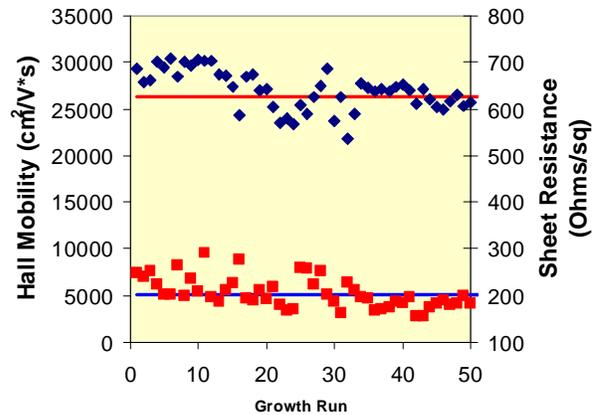
Fig. 4 Statistical process control data for 50 epitaxially grown 3" wafers (Triangles) 300 K electron hall mobility (Squares) sheet resistance.
