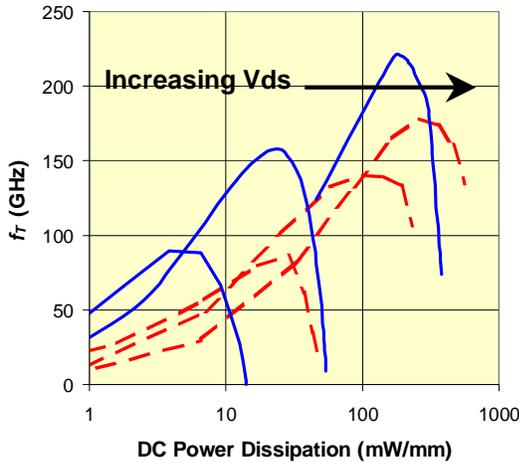
Fig. 8 Extrapolated unity current gain frequency vs. DC power dissipation for AlSb/InAs HEMT (solid) at  $V_{DS} = 0.1, 0.2,$  and  $0.5$  volts and InAlAs/InGaAs HEMT (dashed) at  $V_{DS} = 0.2, 0.5,$  and  $1.0$  volts.
