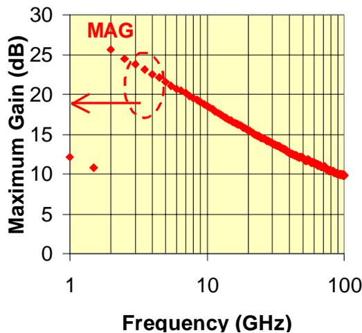
Fig. 7 Measured maximum available gain greater than 10 dB at 100 GHz for 2 x 40-μm devices.
