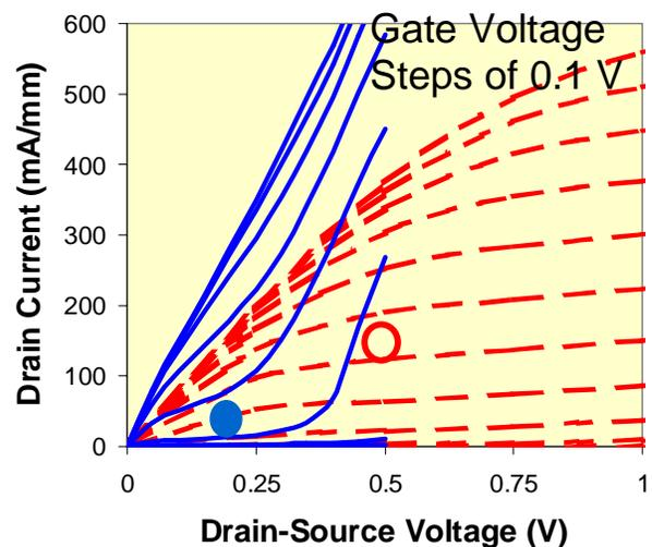
Fig. 1 AlSb/InAs HEMT (solid) bias points for minimum noise figure and lowest DC power dissipation, compared to InAlAs/InGaAs HEMT (dashed). Curves displayed for gate voltage step of 0.1 V.
