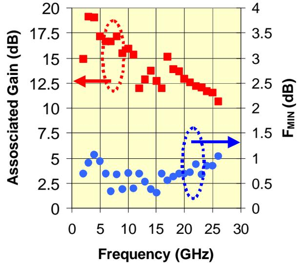
Fig. 9 Measured 2 to 26 GHz associated gain ( $G_A$ ) and minimum noise figure ( $F_{MIN}$ ) at  $V_{DS} = 0.2$  volts and 6 mW/mm DC power dissipation.
