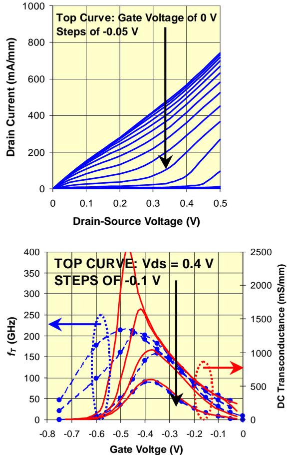
Fig. 5 Top: Measured drain current vs. drain voltage and Bottom: Extrapolated unity current gain frequency (dashed) and measured DC transconductance (solid) vs. gate voltage.
