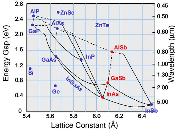
Fig. 2 The  $\text{Al}_x\text{Ga}_{1-x}\text{Sb}_y\text{As}_{1-y}/\text{InAs}$  material system and approximate 6.1 Å lattice constant
