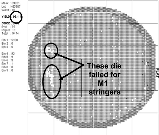
After minor changes in M1 layout to improve the manufacturability of the part without affecting device performance
