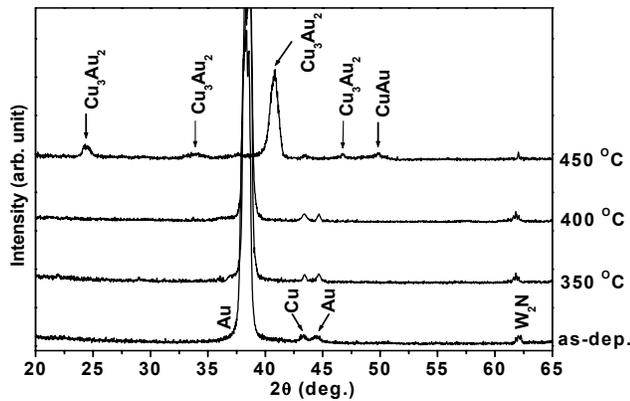
Figure 2. XRDs of Au/WNx/Cu structure with different annealing temperatures
