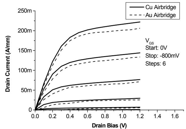
Figure 3. DC characteristics of the devices with copper airbridges and gold airbridges.
