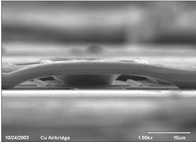
Figure 1. Copper air-bridges on the low noise PHEMT
