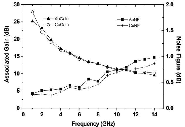
Figure 4. Noise performance of the devices with copper airbridges and gold airbridges
