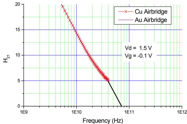
Figure 5. Cut-off frequency of devices with copper and gold airbridge.
