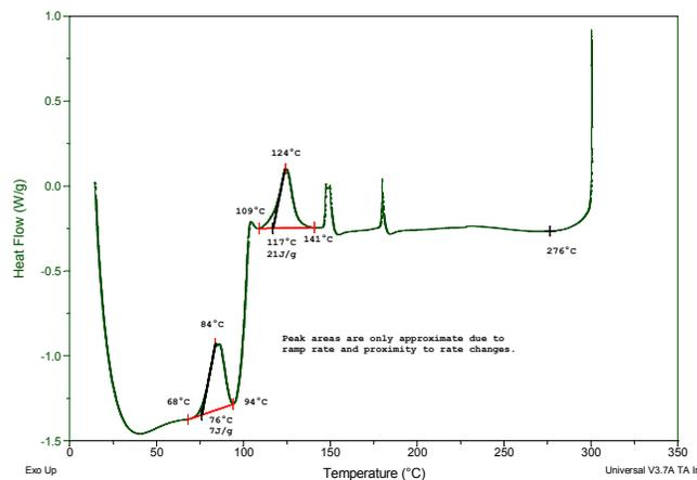
Figure 2. DSC for GenTak™ 330 showing major reaction at 110C and stability through 280C.
