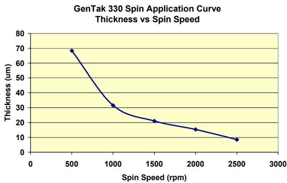
Figure 3. Spin-on thickness vs. speed curve for GenTak™ 330.
