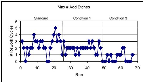
The results from the external descum etch process were significant but further optimizations were needed. Specifically the descum process was being performed on an external RIE descum system. This required unloading the wafers in the middle of an etch run, loading and processing wafers on an external RIE descum system, and finally loading the wafers back into the RIE etch system to finish the etch run. The old and new etch flows are summarized in Table 4.
