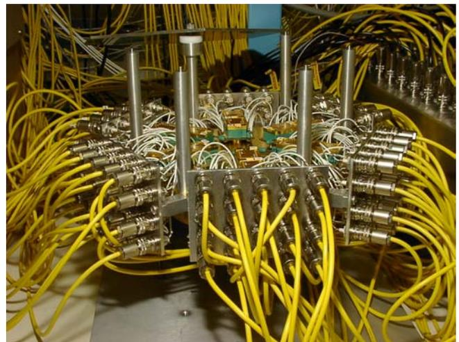
FIG. 7 – THE HEXAGONOL TEST FIXTURE WITH THE PROTECTION COVER OPENED TO REVEAL THE CONSTRUCTION. THE CURRENT MIRROR BOX CAN BE SEEN TO THE RIGHT
