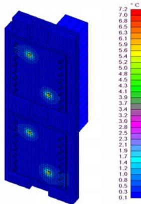
FIG. 5 – THREE DIMENSIONAL THERMAL SIMULATIONS SHOWING THE TEMPERATURE RISE IN THE ZIF SOCKET THERMAL SHUNT.
