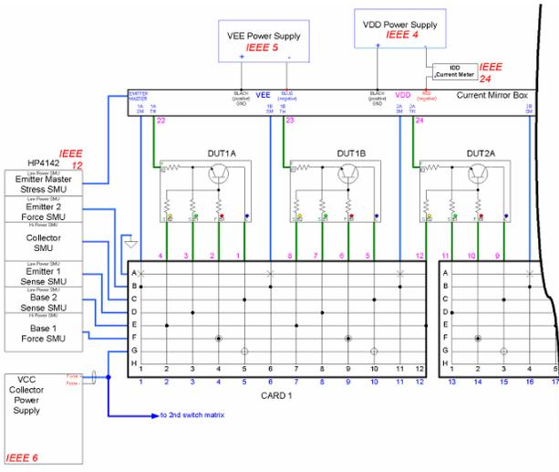
FIG. 4 – A PARTIAL CONNECTION DIAGRAM FOR THAT SHOWS HOW THE SWITCH MATRAICES CONNECT TO THE SMUS, DEVICES, CURRENT MIRROR, AND COLLECTOR POWER SUPPLY.
