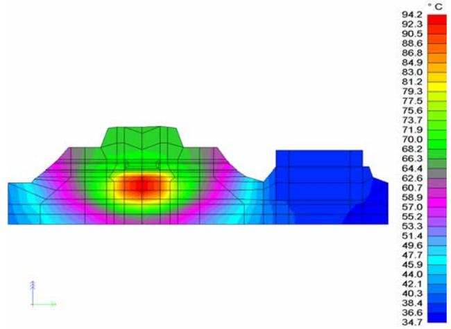
FIG. 6 – THREE DIMENSIONAL THERMAL SIMULATIONS SHOWING THE TEMPERATURE RISE OF A GAAS HBT ON A DIP HEADER IN THE ZIF SOCKET THERM SHUNT AND THE TRANSISTOR JUNCTION.
