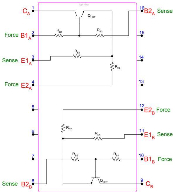
FIG. 8 – THE SCHEMATIC DIAGRAM OF HBT’S MOUNTED ON A DIP HEADER. THE RESISTORS IN THE BASE AND EMITTER REDUCE THE PROCLIVITY OF THE HBT’S TO OSCILLATE. THE DUAL CONNECTIONS PROVIDE FOR KELVIN CONNECTIONS DURING THE MEASUREMENT SEQUENCE.
