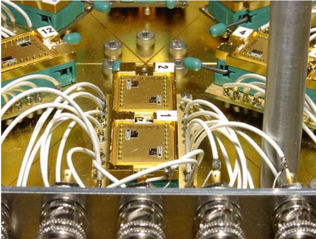
FIG. 3 – ONE PIECE OF THE TEST FIXTURE SHOWING TWO DIP HEADERS ON TOP OF THE THERMAL SHUNTED ZIF SOCKET. EACH DIP HEADER CARRIES A UNIQUE SERIAL NUMBER. THE TEG CHIPS WITH THE HBT'S ARE MOUNTED ON THE DIP HEADER NEXT TO A RESISTOR NETWORK.
