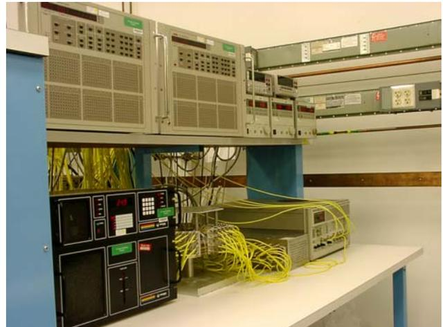
FIG. 2 - THE TWO SWITCH MATRICES, THREE POWER SUPPLIES, CURRENT METER, AND TEMPERATURE METER ARE ON THE TOP SHELF, THE THERMAL CHUCK CONTROLLER, TEST FIXTURE, CURRENT MIRROR, AND SMU'S ARE ON THE BENCH TOP.
