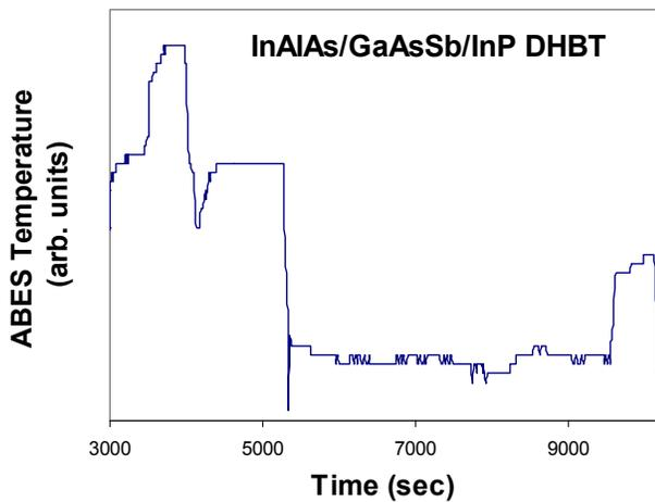
Fig. 4: ABES substrate temperature profile of an InAlAs/GaAsSb/InP DHBT during the growth in Riber 49.
