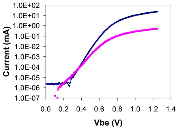
Fig. 6: Gummel plot from InAlAs/GaAsSb/InP DHBT with  $4.5 \times 10^{19} \text{ cm}^{-3}$  base doping.
