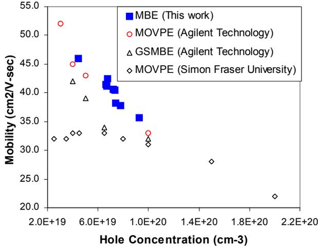
**Fig. 1:** Room temperature hole mobility of CBr<sub>4</sub>-doped GaAsSb as a function of carrier concentration.
