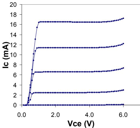
Fig. 5: Common-emitter  $I_c$ - $V_{ce}$  characteristics of a  $50 \mu\text{m} \times 50 \mu\text{m}$  InAlAs/GaAsSb/InP DHBT.
