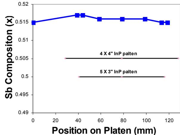
**Fig. 3:** Composition uniformity of GaAsSb vs. radial position across the platens of Riber 49 MBE system.
