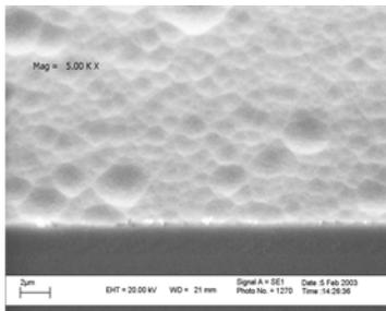
Fig.1. GaAs etched surface with polished starting surface.
