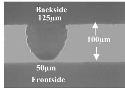
Fig. 11. Cross-section of dry etched,  $100\mu\text{m}$  deep via hole
