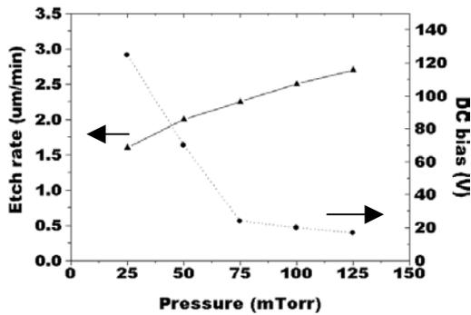
Fig. 5. Variation of etch rate and dc bias with pressure (Power=200W, Time=40min.)
