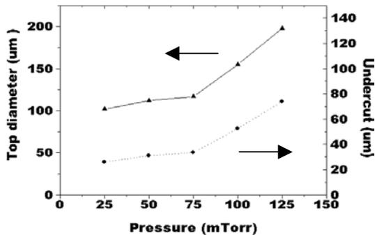
Fig. 6. Undercut obtained as a function of pressure (Power=200W, Time=40min.)
