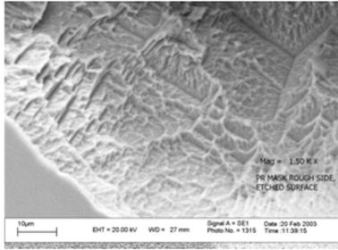
Fig. 9. The surface morphology of via sidewall etched at 200W with photoresist mask
