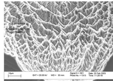
Fig. 7. The surface morphology of via sidewall etched at 200W (Pressure =50mTorr)
