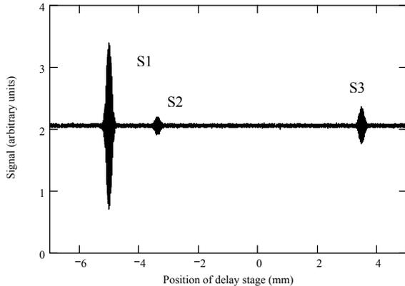
Figure 4: Interferogram of the radiation reflected from multiple quantum well GaAsP/GaP. Features S1, S2, and S3 correspond to reflections from front surface of the sample, MQW portion of the sample and back surface of the sample
