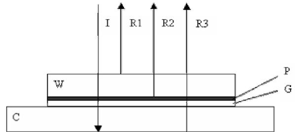
Figure 2: Compound semiconductor wafer W mounted on insulating carrier C by means of wafer gripper G deposited on pattern P carrier C interface. Low coherence beam I is impinging top surface of the wafer W, is partially transparent pattern P, wafer gripper G.
