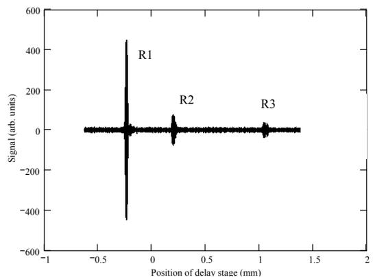
Figure 3: Interferogram of the low coherence light reflected from sample. Features R1, R2, and R3 correspond to reflections discussed in Figure 2.
