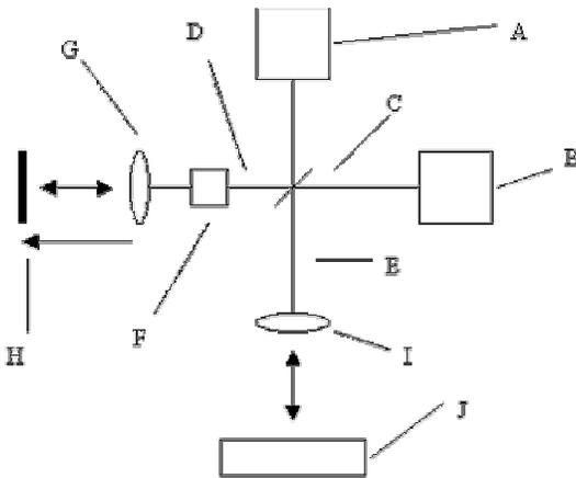
Figure 1: Apparatus used in described experiment comprising of A low coherence source, broad bandwidth infrared source A, detector B, beam-splitter C reference, arm D and signal arm E. Reference arm D comprises of polarization controller F, collimating lens G, and mirror mounted on delay stage H. Signal arm E comprises collimating lens I and sample J.
