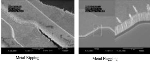
Several reasons were attributed to causing the remaining metal problems. One was poor resist profile attributed to the photolithography process. As the resist profile becomes less re-entrant the area for solvent penetration becomes smaller. The liftoff becomes less effective when there is less solvent penetration. Another reason was the weakness of the solvent. A more aggressive solvent would strip resist faster and more effectively thus overcoming marginal profile situations.
