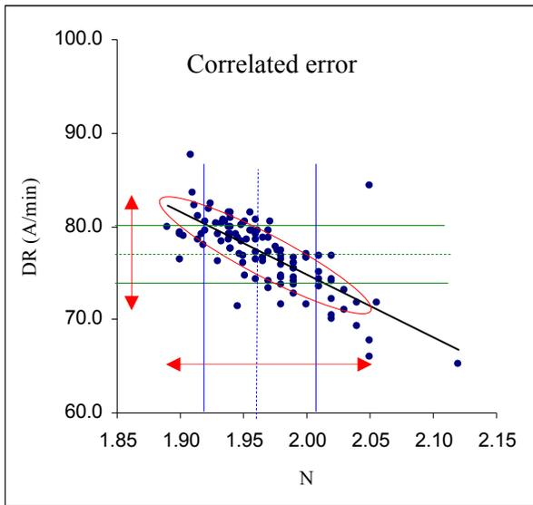
Figure 1 Scatter diagram showing the results of VASE characterization of a-SiN<sub>x</sub>:H samples. Each of the 108 samples was deposited by the same PECVD recipe. The solid lines indicate confidence regions in one- and two- dimensions. The same fraction of points (here 68%) lies - (i) between the two (blue) vertical lines, (ii) between the two (green) horizontal lines, and (iii) within the (red) ellipse. The (red) two-headed arrows show the magnitudes of the correlated errors.
